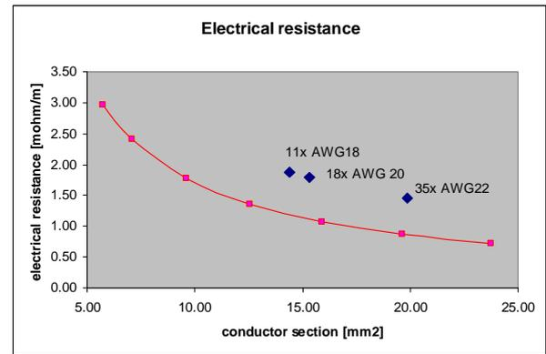
Figure 4 - Comparison of electrical resistance for solid rotor and AWG wires bundles.
