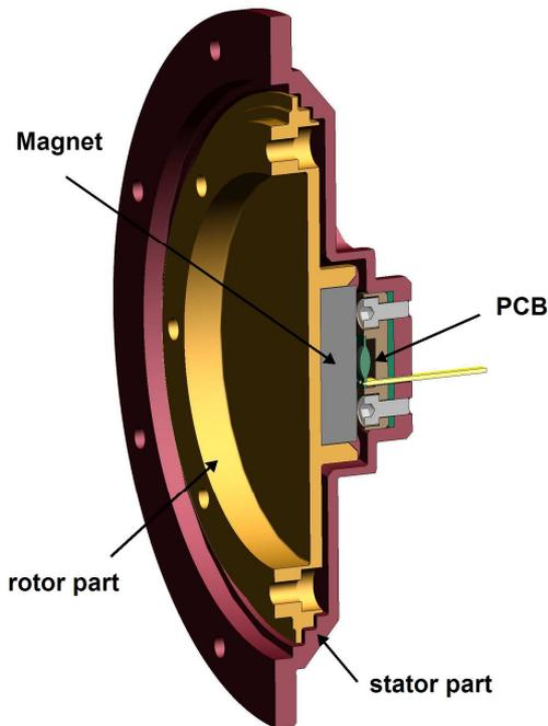
Figure 9 – APS integrated in ASR
