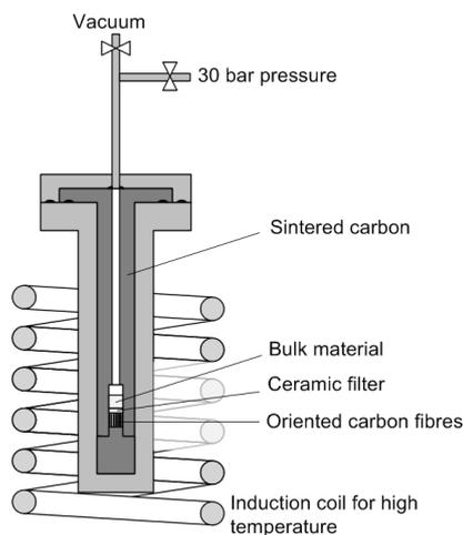
Figure 3 - Composite material test setup
