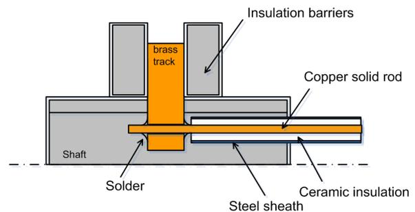
Figure 5 - Solid rod connection
