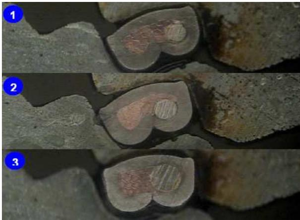
Figure 7 - Splice cross-section
