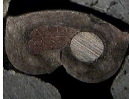
Figure 8 - Splice cross-section
