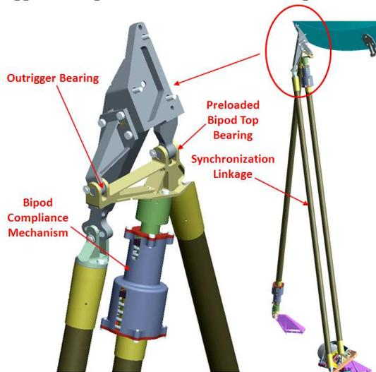
Figure 6: Sync Link & Outrigger Bearing
