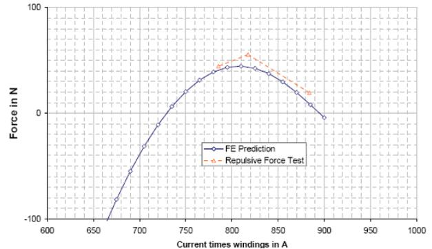
Figure 12 – Repulsive Force vs. Current - Comparison of Measurement & Analysis
