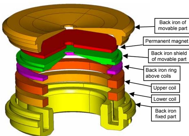
Figure 1 – Parts of URNS HDRM
