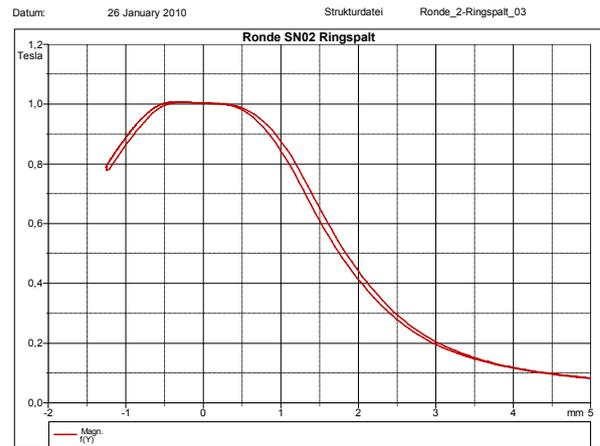
Figure 9 – Measured Magnetic Field inside Gap of Movable Part
