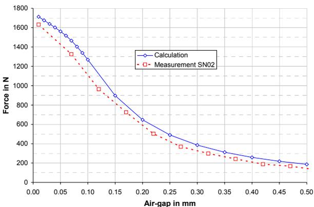
Figure 11 – Force vs. Distance – Comparison of Measurement & Analysis
