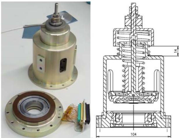
Figure 6 – Test setup of URNS HDRM
