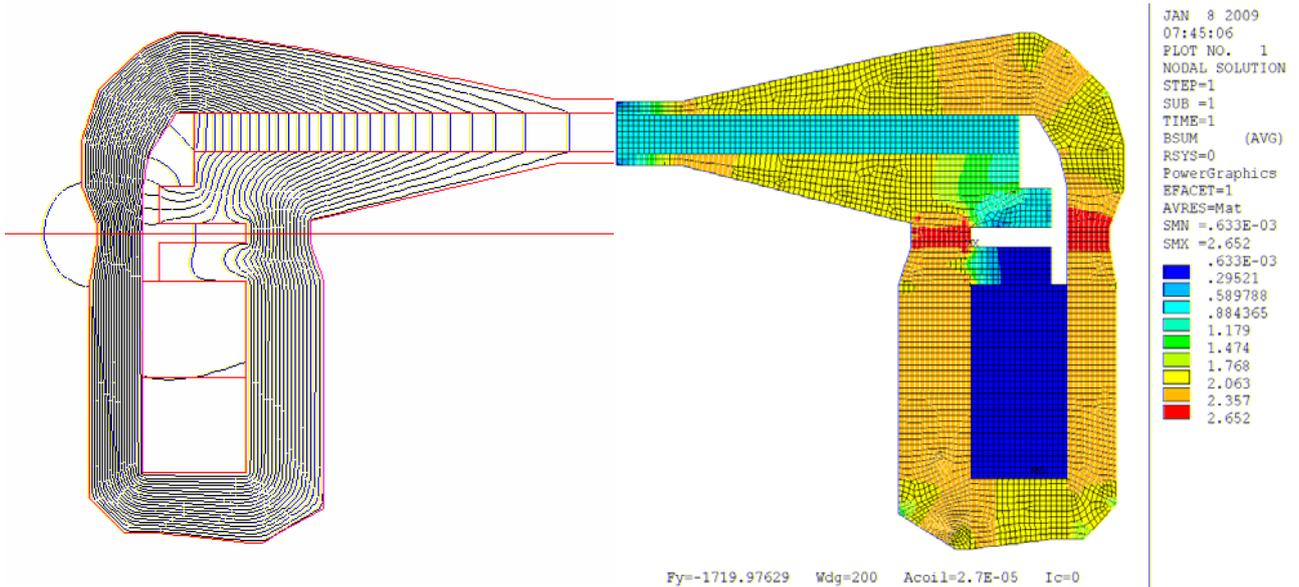
Figure 4 – Static Magnetic Analysis without Current
