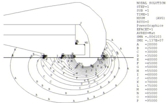
Figure 8 – Calculated Magnetic Field around Movable Part
