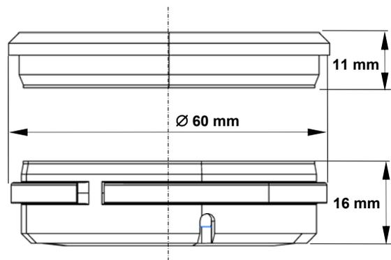
Figure 2 –Dimensions of URNS HDRM
