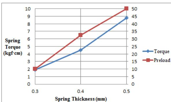
Figure 6. Maximum separable preload according to stiffness of torsional spring.
