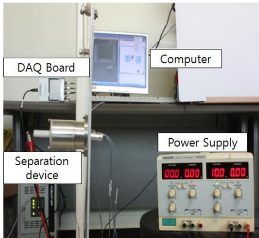
Figure 8. System configuration for shock test
