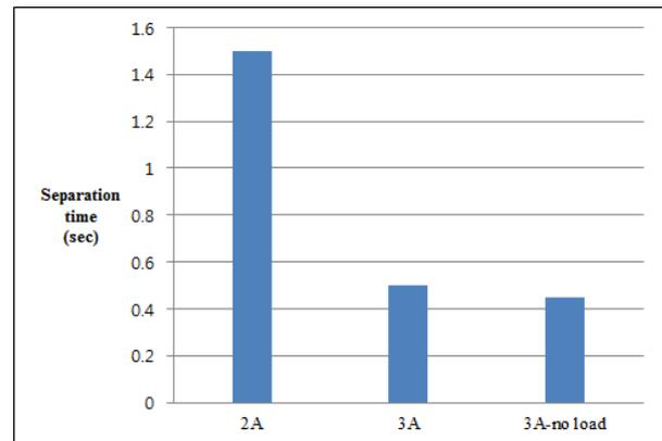
Figure 4. Separation time according to power input and preload.
