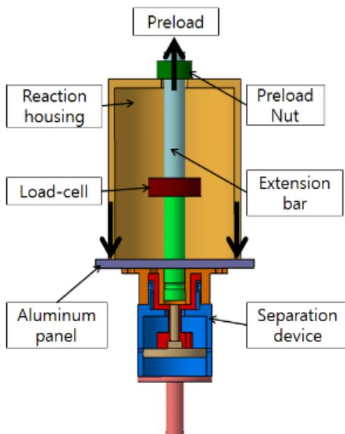
Figure 5. Configuration of preload generator.
