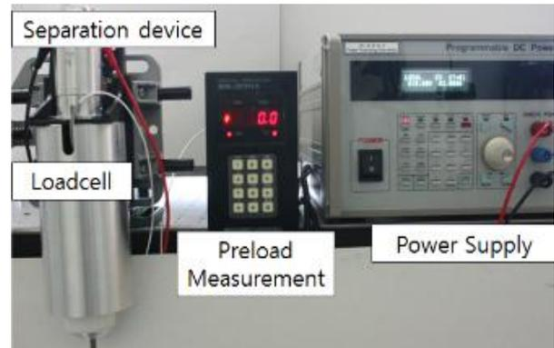
Figure 3. System configuration for separation time test
