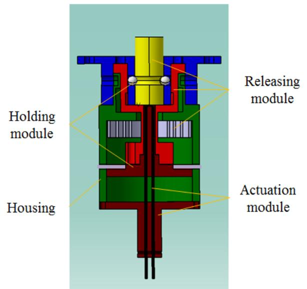
Figure 1. Structure of separation device
