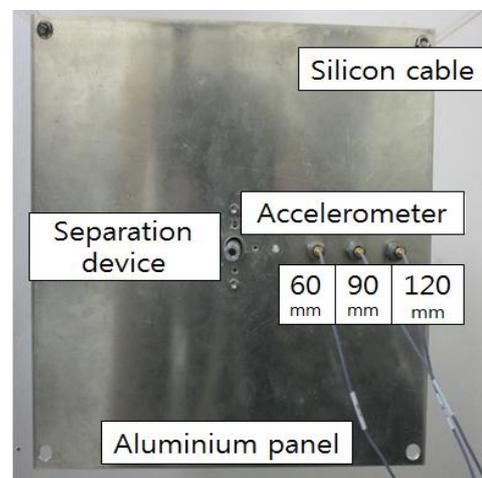
Figure 7. Shock measurement setup on panel
