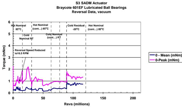
**Figure 6: Accelerated life test results for Braycote601EF (the red curve is the peak torque while the blue curve represents the mean torque)**
