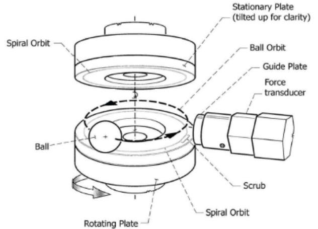
**Figure 1: Spiral Orbit Tribometer test**
