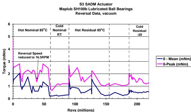
**Figure 7: Accelerated life test results for MaplubSH100b**
