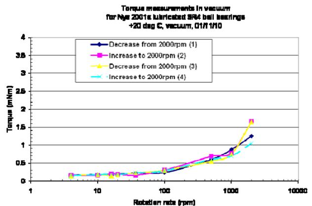
Figure 1: Stribeck curves measured at 20 deg C (cold case)
