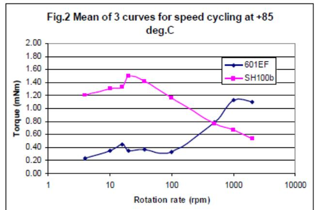
**Figure 5: Stribeck curves measured at 85 deg C for Braycote and Maplub**
