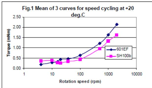
**Figure 3: Stribeck curves measured at 20 deg C for Braycote and Maplub**
