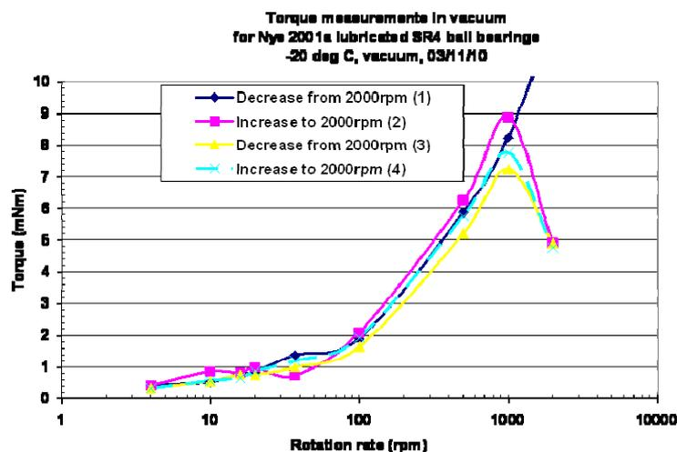
Figure 2: Stribeck curves measured at -20 deg C (minimum temperature)
