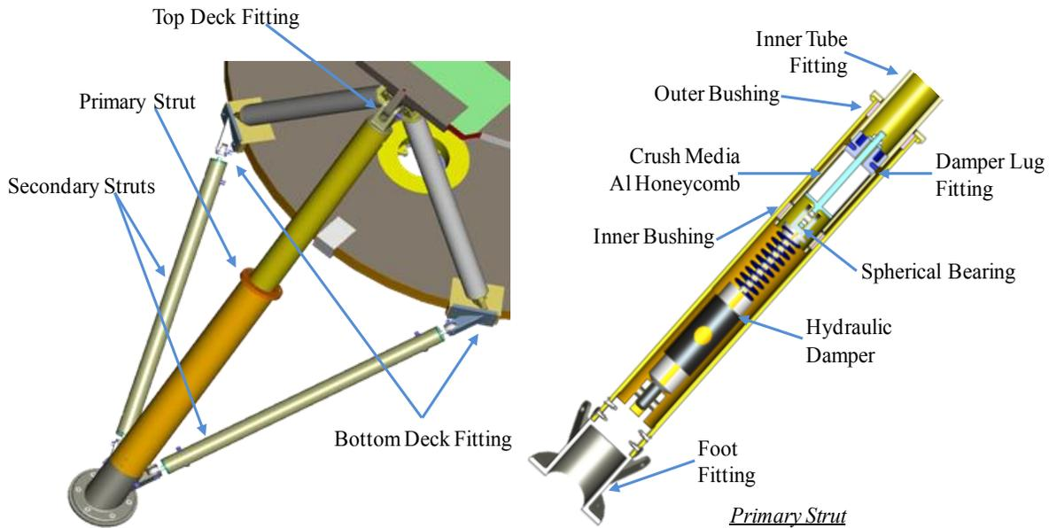
Figure 2. Leg Assembly Details
