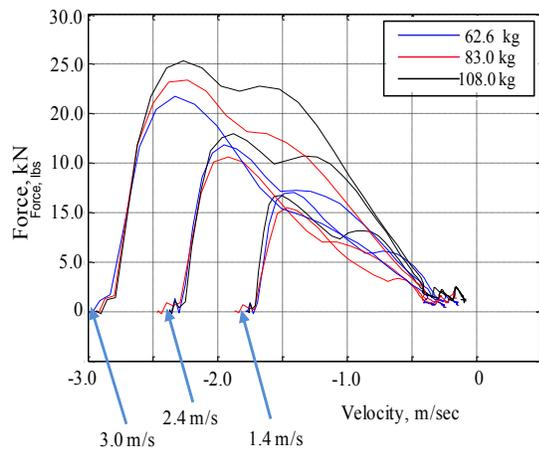
Figure 7. Hydraulic Damper Performance Curves
