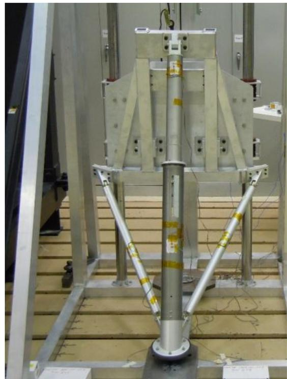
Figure 8. Leg Assembly Impact Test
