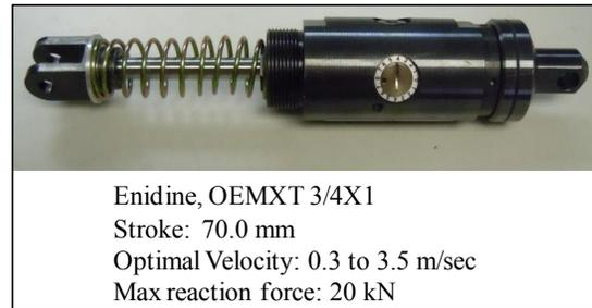
Figure 3. Hydraulic Damper
