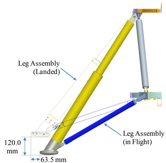
Figure 4. Leg Assembly in Flight and Landed Configurations
