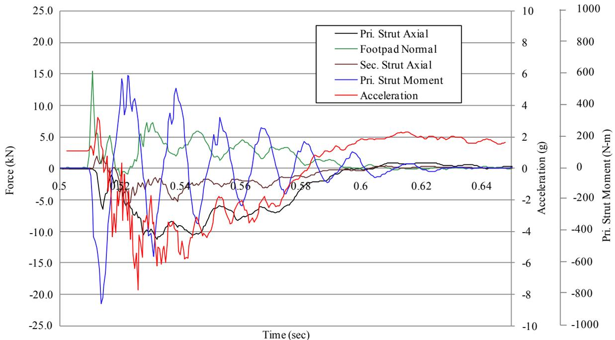
Figure 9. Leg Assembly Test Results - Loads and Acceleration Velocity of 3.0 m/sec
