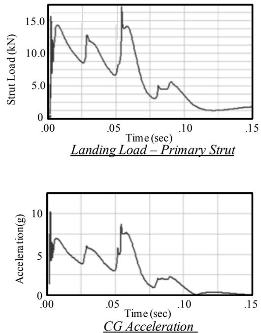
Figure 5. Results of Dynamic Analysis for Impact Velocity of 4 m/sec
