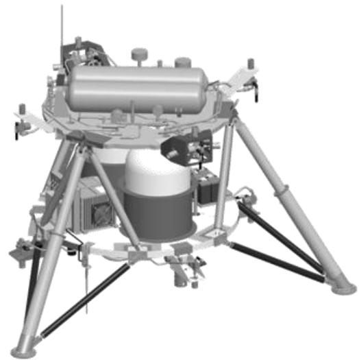
*Figure 1. Warm Gas Test Article*
