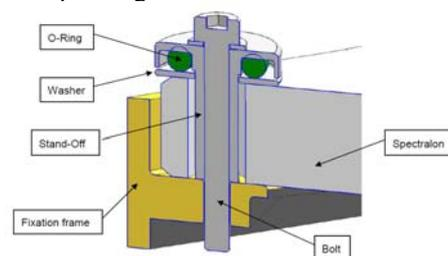
Figure 7. Sectional view of Spectralon plate fixation
