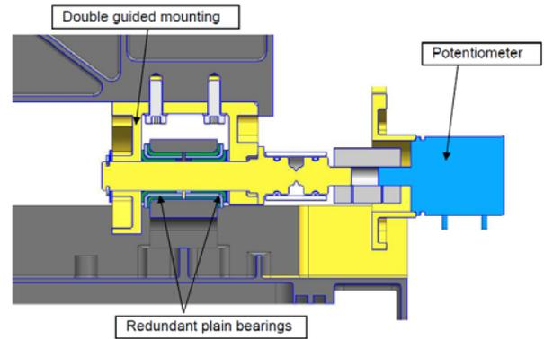
Figure 12. Separation Mechanism.
