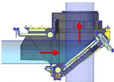
Figure 3. Cutaway view of the mechanism (Sun calibration mode)
