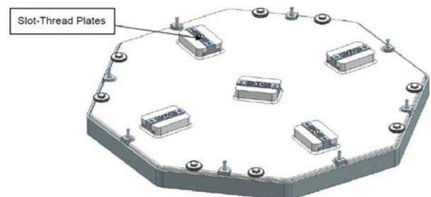
Figure 8. Spectralon Mounting Plate.
