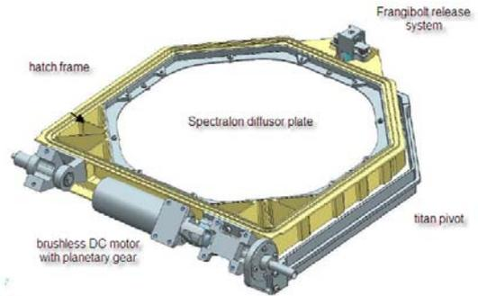
Figure 5. CAD view of the sun diffuser hatch (SDH)
