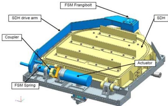
Figure 9. The Fail Safe Mechanism (FSM).
