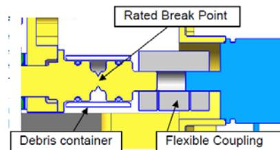
Figure 13. Rated Breaking Point of Potentiometer Axis
