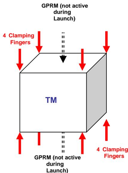
Fig 3. CMLA Clamping Principle
