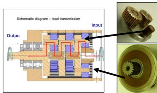
Fig 12. Ti Gear equipped with Bronze Planets and Vespel<sup>®</sup> bushings/spacer
