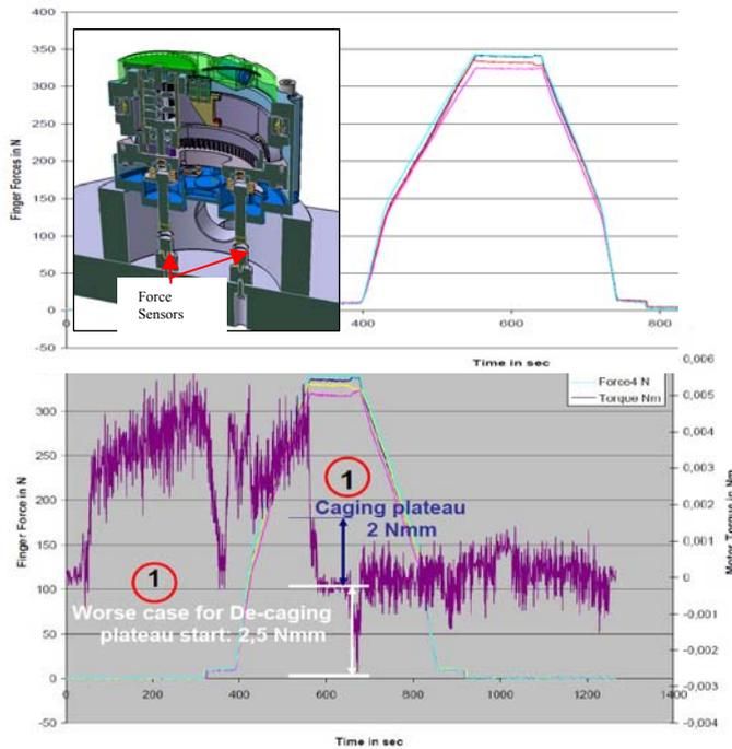
Fig 18. CMLA Caging/De-Caging Torque (NM) vs. caging forces
