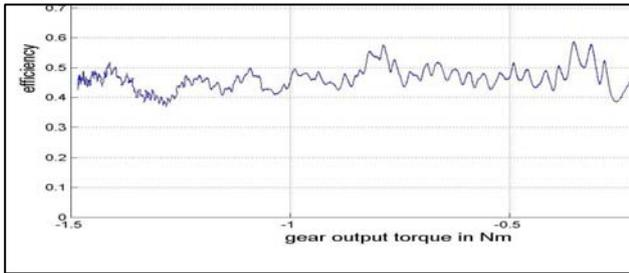
Fig 13. Planetary Gear Efficiency
