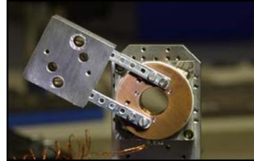
Fig 11. Piezo Motor during torque/life test
