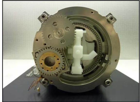
Fig 16. CMLA Integrated, top view, with GPRM dummy in the centre (white element)
