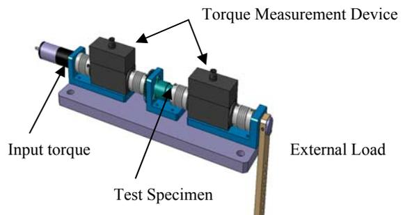
Fig 17. Gear efficiency Test Setup
