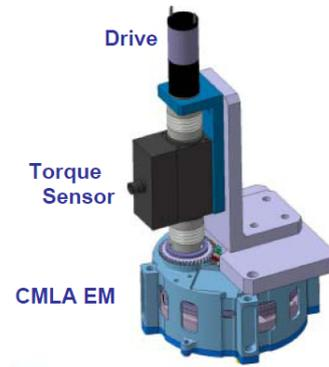
Fig 19. CMLA Torque measurement set up
