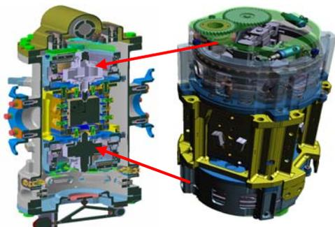
Fig 2. LTP Inertial Sensor and CMLA (2 Halves)
