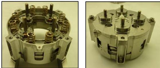
Fig 15. CMLA during Integration and Integrated
