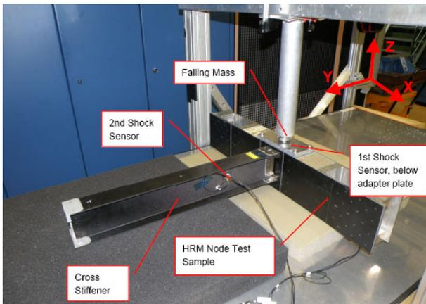
Figure 11: HRM Transfer Function Test Sample
