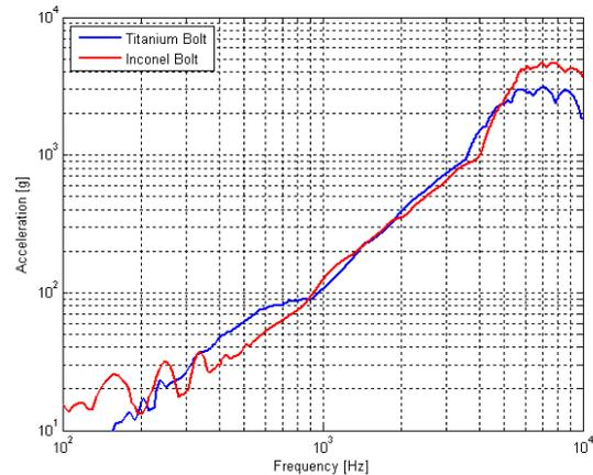
Figure 9: SRS comparison Titanium - Inconel Bolt
