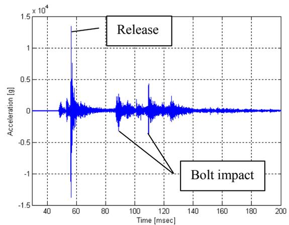
Figure 13: Shock Time Signal
