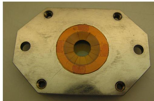
Figure 7: Kapton particle seal
