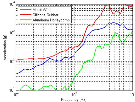
Figure 6: SRS Results of different Shock Dampers
