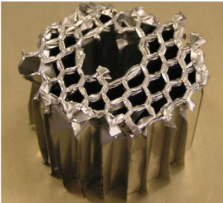
Figure 5: Pre-crushed honeycomb
