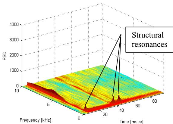
Figure 15: SRS at Electronics Level
