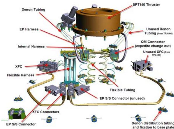
Figure 2: EP Subsystem for SPT140
