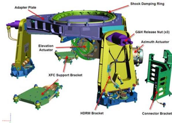
**Figure 3: Common Lower Structure**
