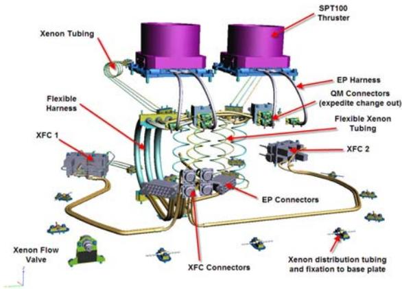
Figure 1: EP Subsystem for SPT100
