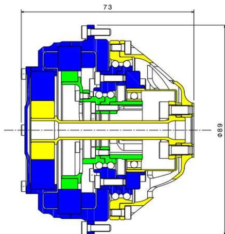
Figure 6. Actuator cross section
