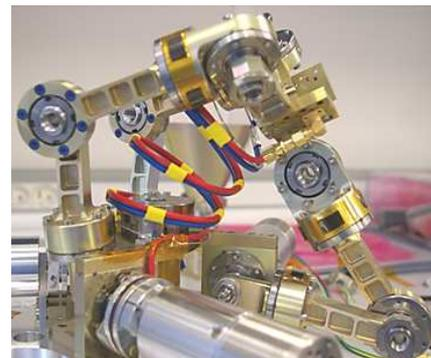
**Figure 5. Breadboard of RF cable routing**
