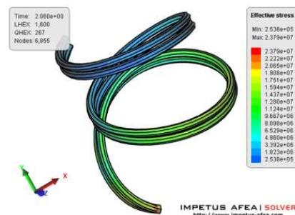
Figure 10 : RF harness Simulation
