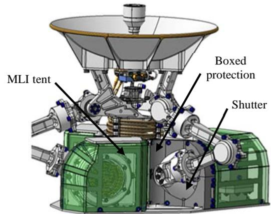
Figure 8. Thermal protection on the base plate.
