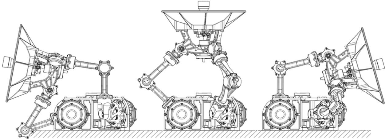
Figure 1. The antenna pointing system 3POD
