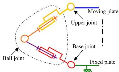
**Figure 3. 3POD schematics and Mechanical linkage of one 3POD leg**
