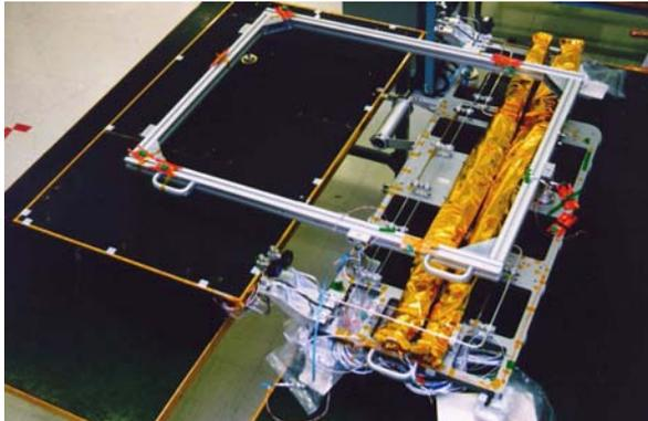
Figure 9. DELPHRAD Deployable Radiator
