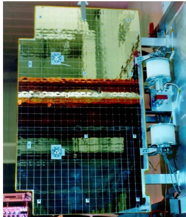
Figure 8. STENTOR Deployable Radiator
