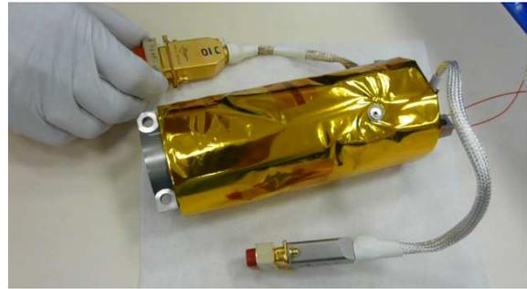
Figure 5. SMA cartridge
