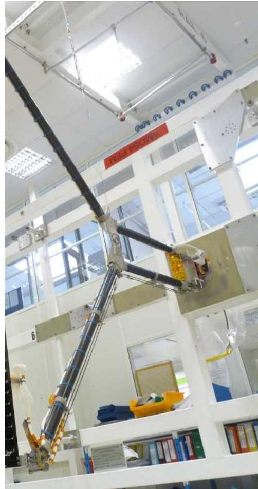
Figure 1. Solar Array with its SMA root hinge
