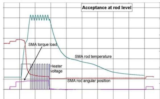
Figure 13. Motorization test at SMA actuator level
