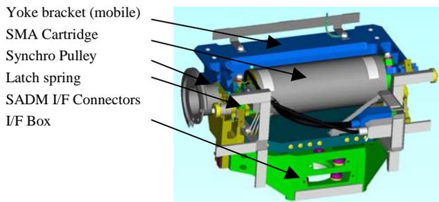
Figure 2. Solar Array root hinge main parts
