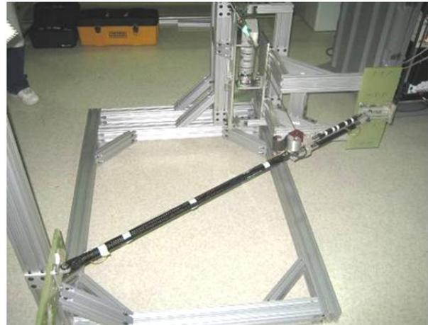
Figure 4: PWDA Strut installed on Torque Test Equipment in Deployed Configuration
