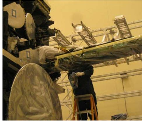
Figure 17: Technician Preloading an LRA
