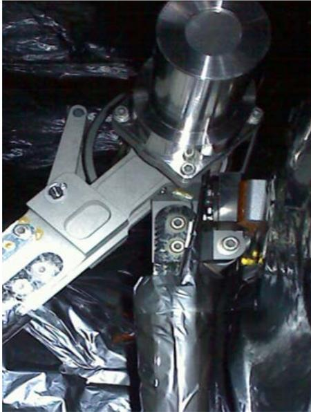
Figure 16: Strut Fully Stowed in the Strut Guide as seen by the Camera
