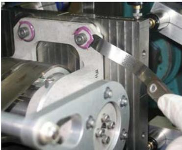
Figure 9: Hinge Shearsert with Failed Epoxy Bondline
