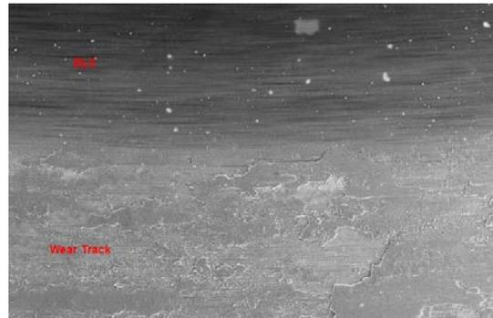
Figure 7: Wear Track on Axle of Damper Gear
