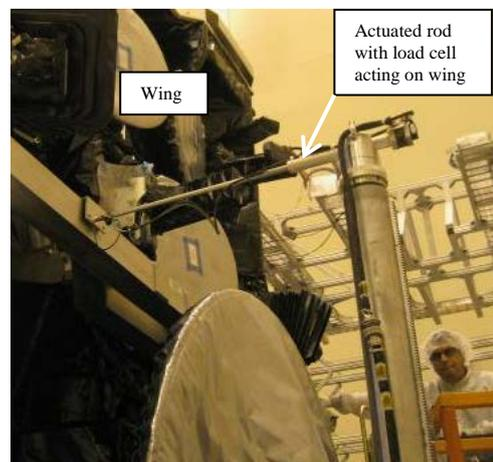
Figure 18: Hinge Characterization Test Setup
