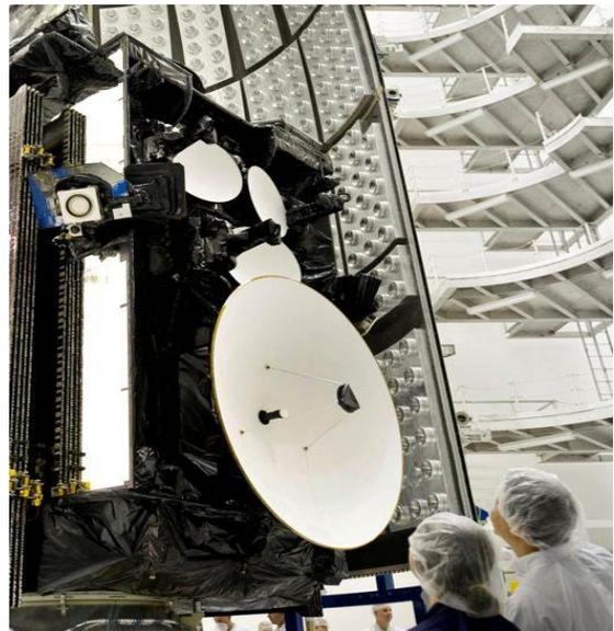
Figure 21: Payload Wing installed on the Vehicle and Encapsulated in the Rocket Fairing.
