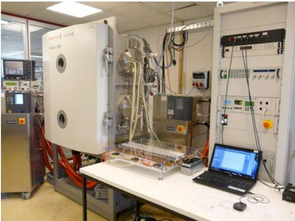
Figure 19. Functional and voltage breakdown test bench (TVAC and interfaces)
