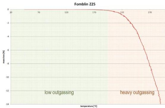
Figure 5. Mass loss of Fomblin Z25 in thermal vacuum. Temperature increased at 1°C/min
