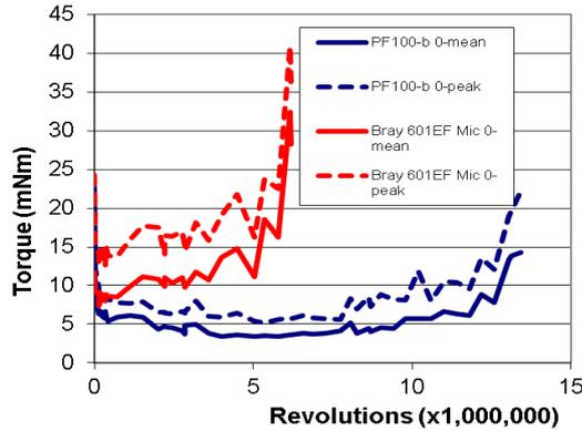
Figure 13: PFPE grease comparison on ball bearing
