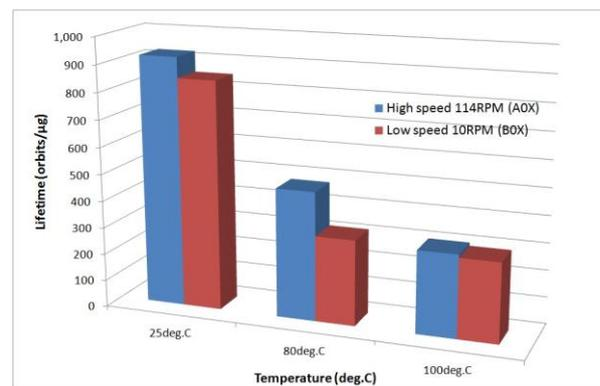
Figure 4. Lifetime comparison of tests performed at 1.50GPa peak, at varying speed
