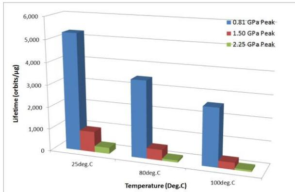
Figure 2. Lifetime results of SOT, showing dependence of life on contact stress for all temperatures
