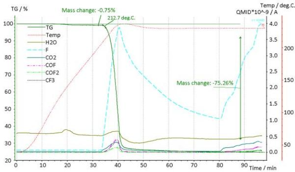
Figure 10. PFPE + FeF<sub>3</sub> heated from 40°C to 230°C with 1 hour of isothermal step.
