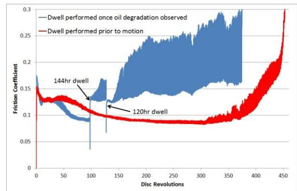
Figure 12. Dwell test on POD, showing increase in friction following 144hr dwell, once degradation of oil initiated through sliding
