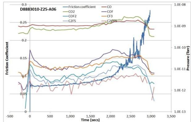
Figure 7. Friction and volatile gas evolution at 80°C, 2.25GPa
