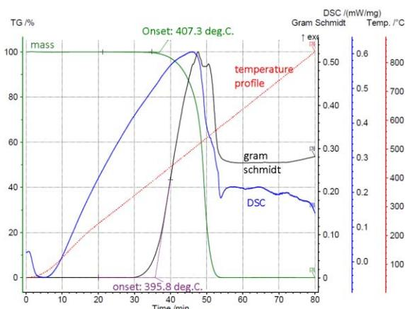
Figure 8. Pure PFPE heated in N<sub>2</sub>.
