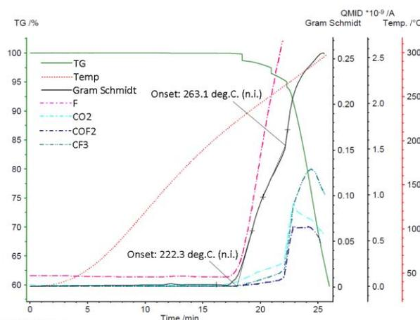
Figure 9. PFPE/FeF<sub>3</sub> heated in N<sub>2</sub>.
