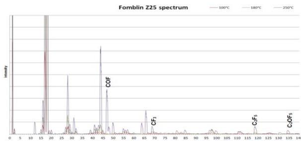
Figure 6. RGA spectrum of Z25 during sublimation test, taken at various temperatures
