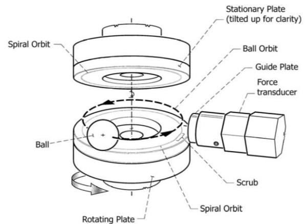
Figure 1. Internal arrangement of SOT
