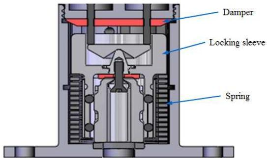
Figure 2: Model 9421 Cross section.
