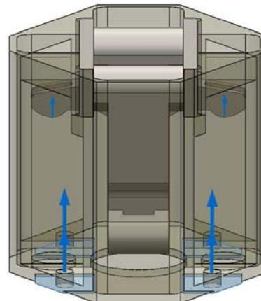
Figure 23: Load on Housing and Tension Shaft
