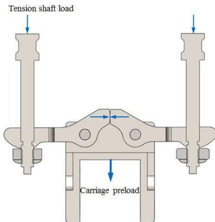
Figure 6: Collapsible Rocker Arms - Armed
