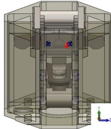
Figure 22: Pin joints definition in Y-Z plane
