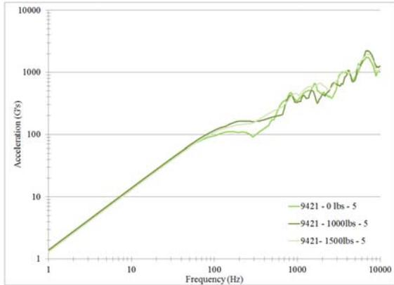
Figure 20: SRS of 9421 Actuator at various loads
