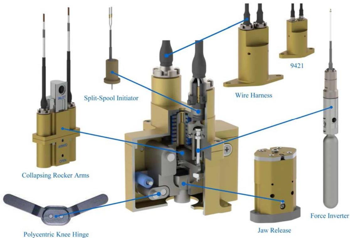
Figure 1: Design Concept Cut View
