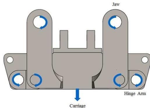
Figure 8: Polycentric Hinge Design
