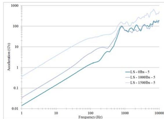
Figure 19: SRS of Low Shock Non-Explosive Actuator at various loads
