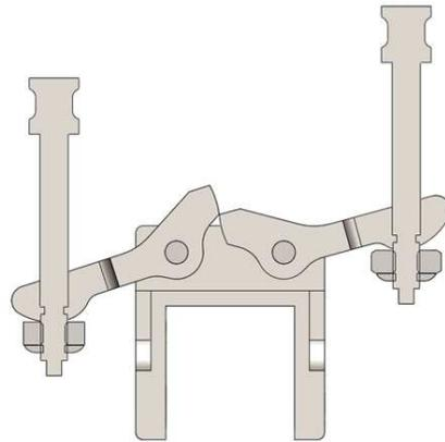
Figure 7: Collapsing Rocker Arm - Initiated
