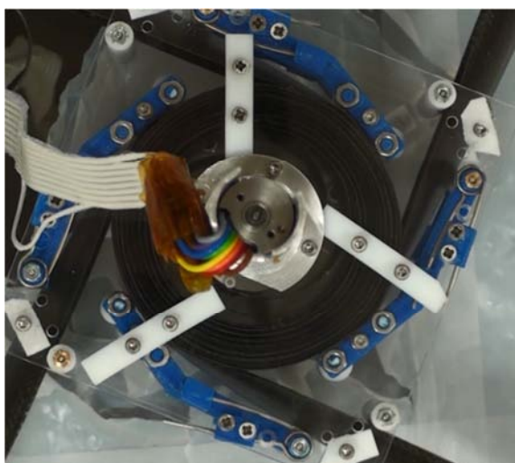
Figure 12: blossoming of the CFRP coil during boom deployment. As the coil expands due to relative motion of the coiled booms, a gap appears between the spindle and coil.
