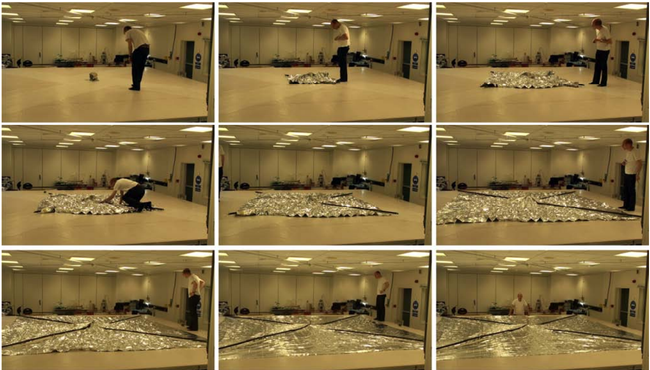
Figure 15: Successful sail deployment test with the CFRP booms. The sail deployment table is covered with an anti-static Sentrex film, and the booms are suspended from a cross-shaped gantry attached to the ceiling at the tip and mid-length points.
