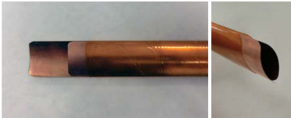
Figure 4: two CuBe tape springs face each other to form a lenticular cross-section; a Kapton sheath provides improved torsional stiffness, while enabling the tape springs to slide with respect to each other as the booms are coiled.
