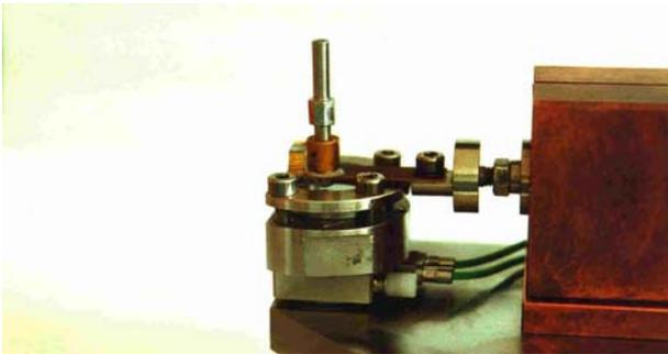
Figure 1: Fretting device: Detail showing the fixation of pin (upper rod) and disc (mounted directly on a force transducer).
