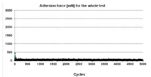
*Figure 5: Adhesion as function of cycles between SS17-4PH with pre-treatment and MoSx/WC coating in contact to PH15-5PH pin (1cycle = 2000revs)*
