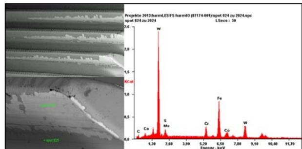
Figure 14: Loaded tooth flank of FS after test. Top left and bottom left: SEM image of FS tooth, right: EDX spectra within contact zone
