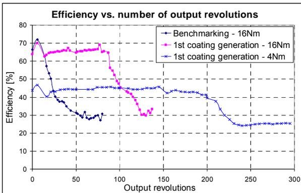
Figure 12: Course of efficiency for testing of first dry lubricated HD gears
