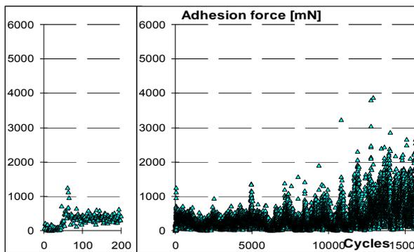
Figure 2: Adhesion force as function of cycles: Detail on the left shows that lubrication of pure  $\text{MoS}_2$  is lost after 50 cycles = 100.00 revolutions (1 cycle = 2000revs).
