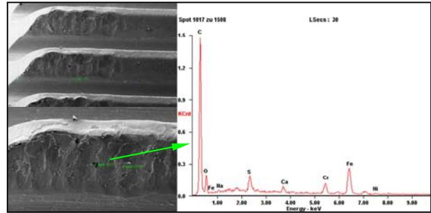
Figure 13: Loaded tooth flank of FS after test. Top left and bottom left: SEM image of FS tooth, right: EDX spectra within contact zone
