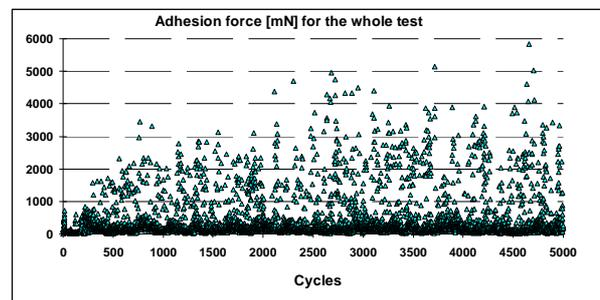
*Figure 4: Adhesion as function of cycles (1cycle=2000revs) between SS17-4PH with pure MOS2 coating in contact to blank PH15-5PH pin*
