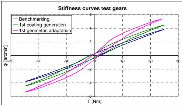
Figure 11: Stiffness curves gears for Benchmarking, 1st coating generation and 1st geometric adaptation
