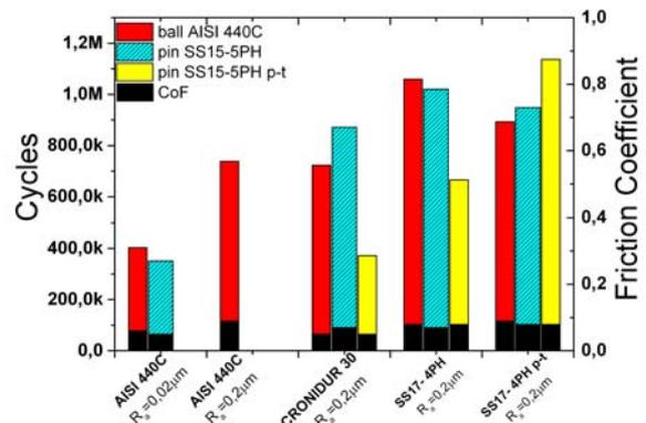
Figure 3: Endurance and average CoF of the  $\text{MoSx-WC}$  coating measured on the different pin-on-disc tests. Coating reference:  $\text{MoSx-WC}$  (25988,  $\sim 1.9\mu\text{m}$ ). Substrates: AISI 440C (polished); 440C, CRONIDUR<sup>®</sup>30, SS17-4PH and SS17-4PH with pre-treatment ( $R_a = 0.2\mu\text{m}$ ). Pin/ball: AISI 440C, SS15-5PH, SS15-5PH with pre-treatment (polished).
