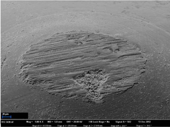
Figure 6: Contact zone of pin SS15-5PH after test to MoSx/WC coating showing a well developed tribo-layer
