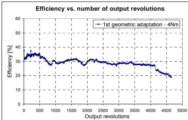
Figure 15: Course of efficiency of dry lubricated Harmonic Drive® gears with 1st geometric adaptation.
