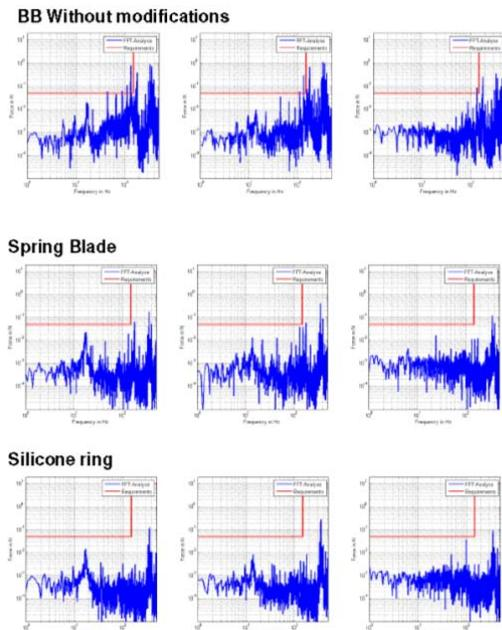
Figure 14: Micro Jitter disturbance forces
