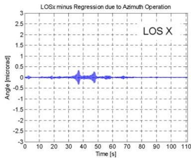
Figure 3: Improved LOS micro vibration
