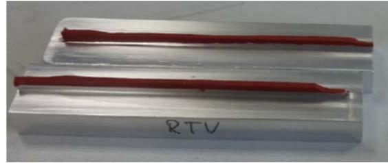
Figure 9: Failure mode of shear samples
