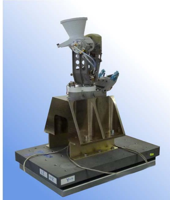
Figure 15: Jitter test setup for APM
