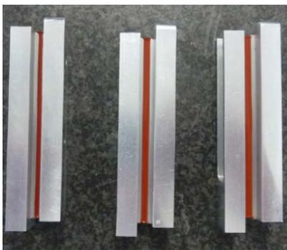
Figure 8: Longitudinal shear samples
