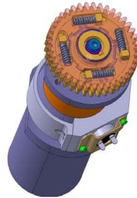
Figure 4: Original FM design of APM actuator link which was planned to be modified
