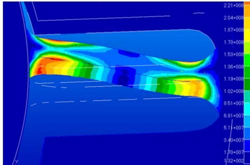
Figure 7: FEM stress in spring blade
