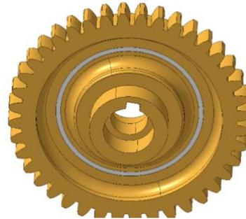
Figure 5: GW with silicon ring
