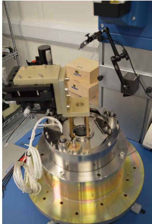
*Figure 6. GSE Lens Installation with- Opticentric MOT300 with Focus Mechanism on Tip-Tilt Table*
