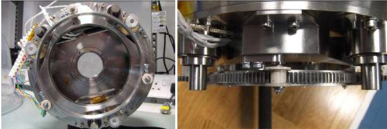
Figure 10. Guide Roller Module Installed on EM Focus Mechanism
