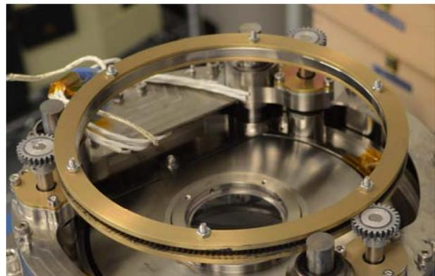
Figure 5. Gear and Pinion Assembly
