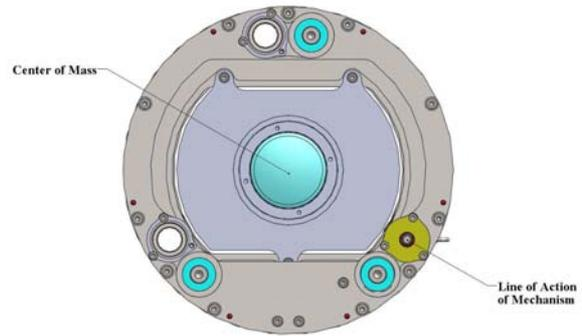
Figure 4. Single Screw Configuration – Moment Load
