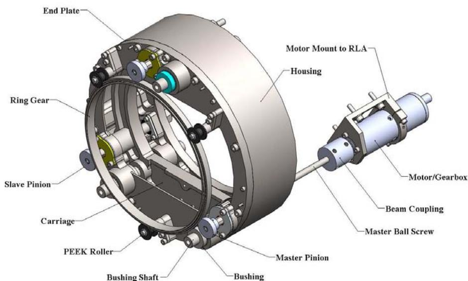
Figure 3. PFM Focus Mechanism Components
