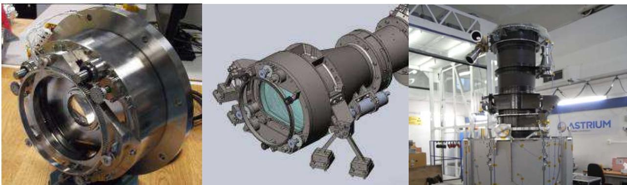
Figure 1. DMC3 Imager Focus Mechanism EM (L), PFM Model with RLA Assembly (C), and RLA Mass Dummy on SQM Imager at top right (R)
