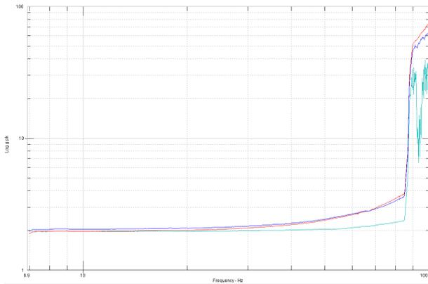
Figure 7. Plot of Z Axis (Optical Axis) Sine Response – Single Screw Variant Sees 82g, Abort!
