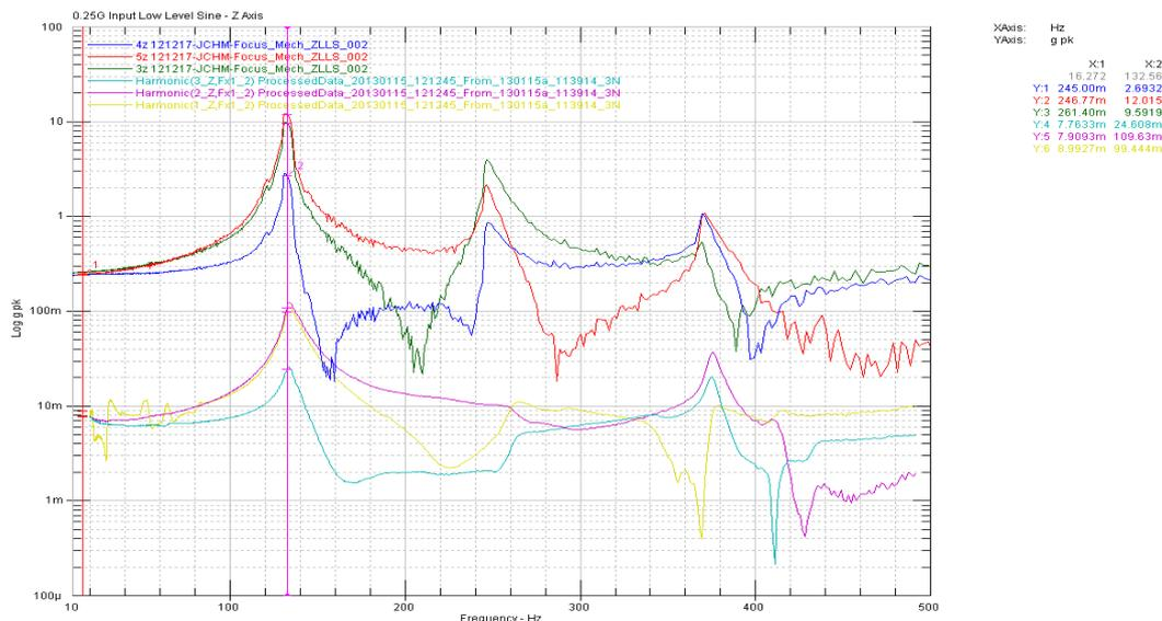
Figure 9. Low Level Sine Sweep and Stinger Responses – First Modes Coincide
