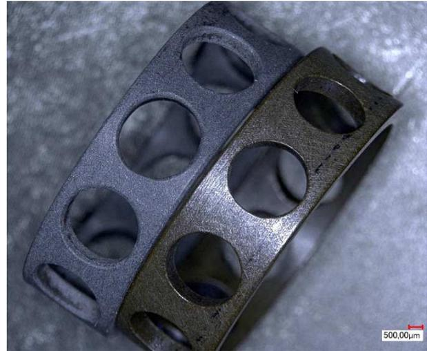
Figure 2: Cages (left side: PGM-HT, right side: Vespel SP3)
