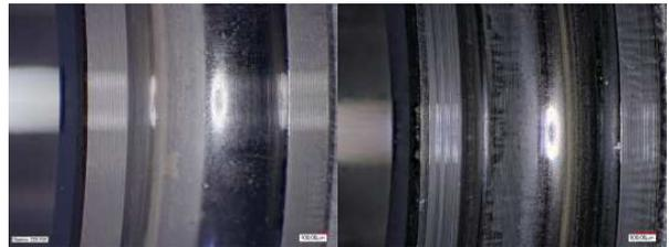
Figure 11. Bearing race after test, Left side: No. 6 (MoS<sub>2</sub>-B); Right side: Nr 3 (MoS<sub>2</sub>-E)
