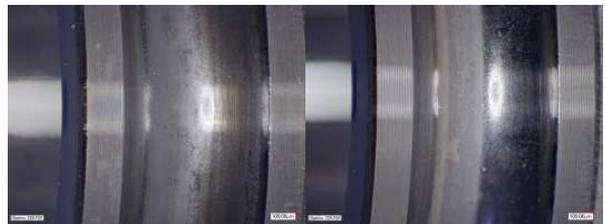
Figure 12. Bearing race after test, Left: Bearing No. 1 (Si<sub>3</sub>N<sub>4</sub>-balls) Right: No. 6 (AISI 440C-balls)
