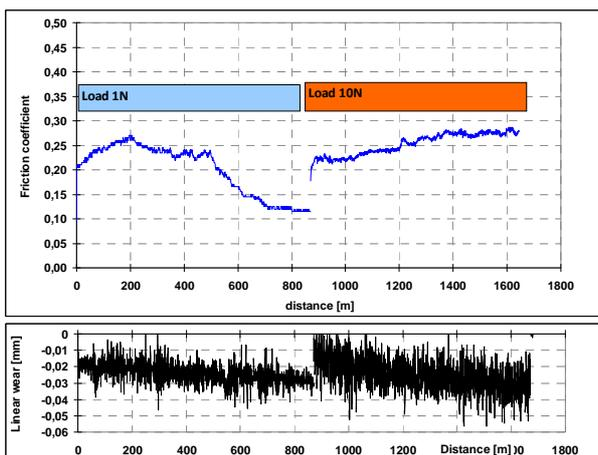
*Figure 9: Composite C02 (..20GF..): Super-low-friction at low loads disappears after increase of load. Linear wear is high for higher load (steeper slope on the right)*
