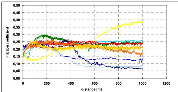
Figure 9: Ref-Material-F1: Friction as function of test duration, high friction in N2.
