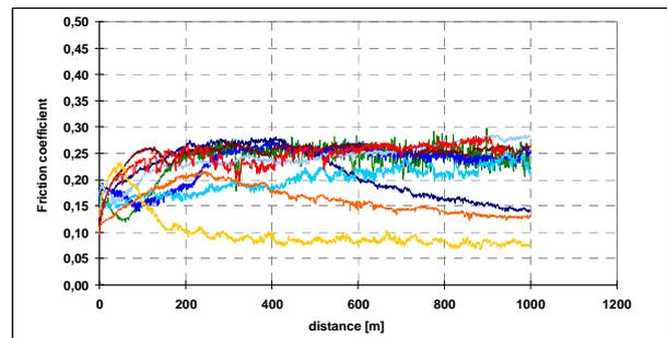
Figure 2 Composition C01 (.25GF..): Friction as function of test duration, partly super-low-friction for low load and at 80°C.
