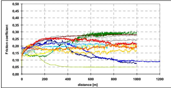
**Figure 3:** Composition C02 (..20GF..): Friction as function of test duration, partly super-low-friction for low load/high speed and high load/low speed (all at RT).
