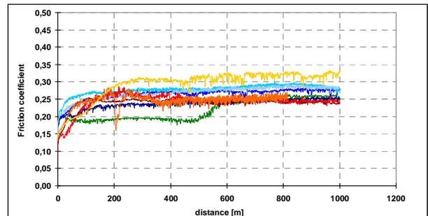
**Figure 8:** Composition C10 (..10CNF..): Friction as function of test duration, using CNF without  $\text{MoS}_2$
