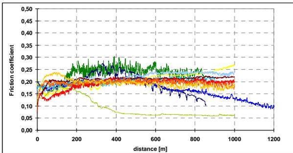
**Figure 5:** Ref-Material-P2: Friction as function of test duration, partly super-low-friction for low load/high speed and high load/low speed (all at RT), similar to C02.
