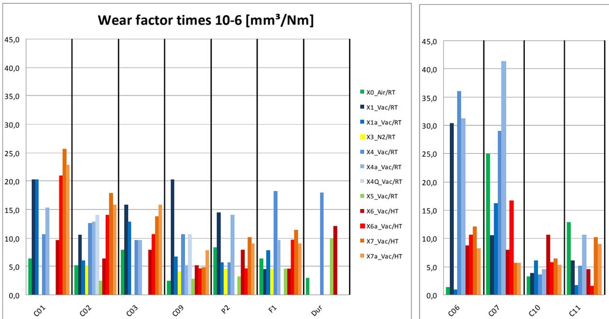
Figure A2: Pin-On-Disc tests: Wear factor (calculated from wear diameter on pins after test, error of measurement about +/-1): These higher loads (5N) were also used in reference tests [11]. (Speed 0.1 m/s and 0,01m/s for series X5 only, counter material AISI440C). (Data for Duroid (“Dur”) estimated from images in [11] tested against AISI52100.)
