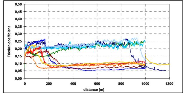
**Figure 6:** Composition C06 (...25SiO2...): Friction as function of test duration, super-low-friction in almost all tests.
