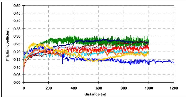
**Figure 4:** Composition C03 (..15GF..): Friction as function of test duration, super-low-friction not clearly identified (low load at RT).
