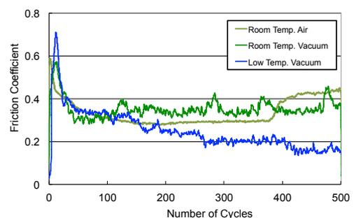
Figure 8. Friction behaviors of brake materials under different conditions.
