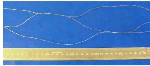
Figure 2. Photograph of a net-type tether.
