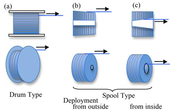
Figure 3. Types of tether deployment systems.
