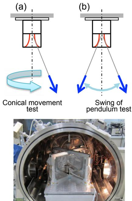
Figure 9. Durability tests for the tether installation part. (a) Conical movement test, (b) Swing of pendulum test.
