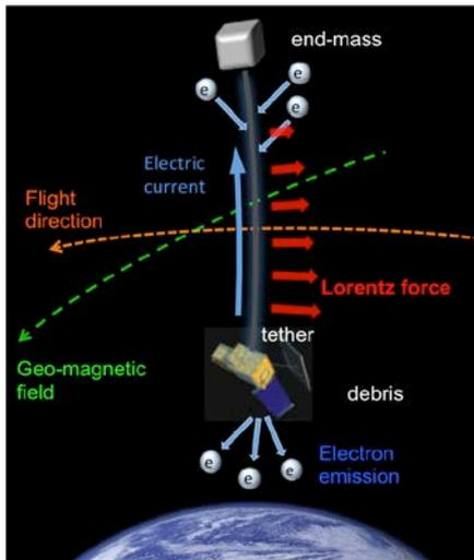
Figure 1. Conceptual image of demonstration of an EDT debris removal system.
