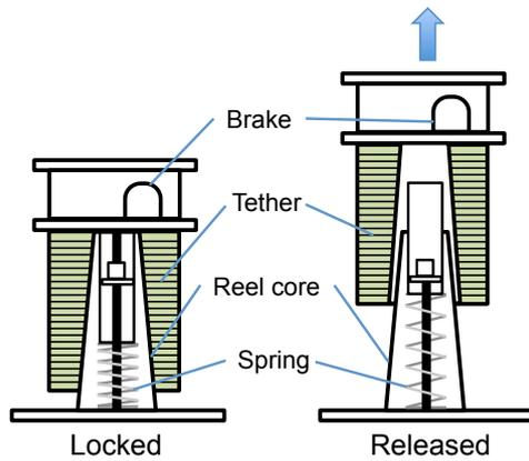
Figure 5. Schematic drawing of tether release systems.
