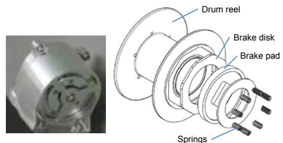
Figure 7. Schematic diagram of brake systems.
