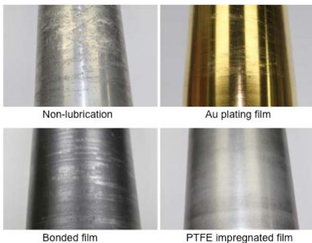
Figure 6. Surfaces of reel cores after a vibration test and pulling out from a rolled tether.
