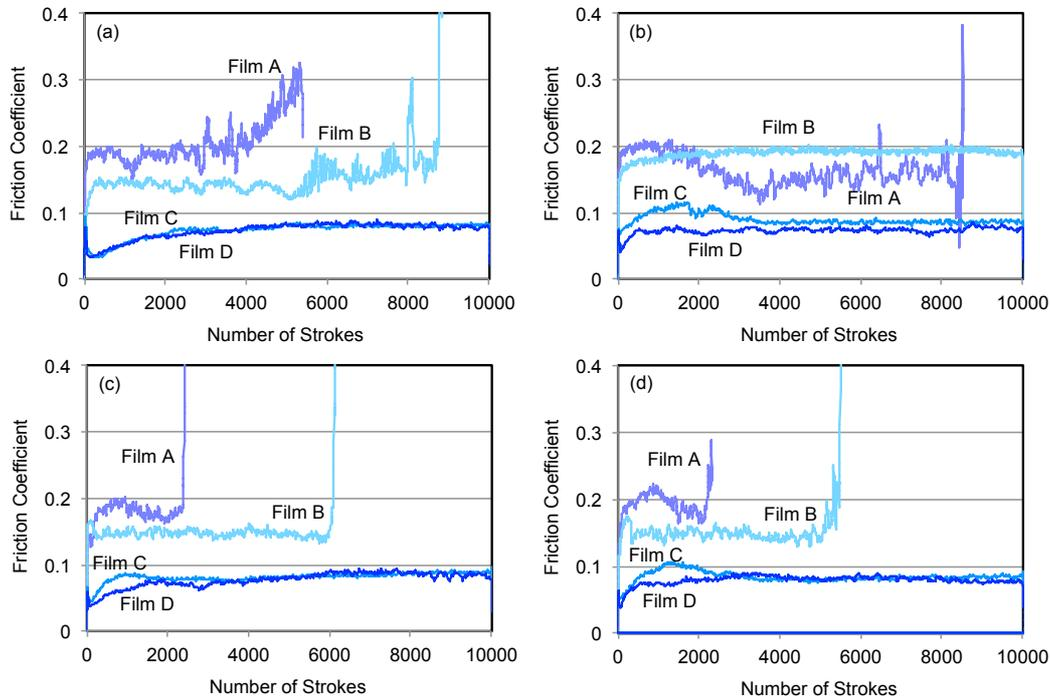
*Figure 4. Friction behaviors of tested bonded lubricant films with different substrates and counterparts. Substrate/Counterpart: (a) stainless steel/ stainless steel, (b) stainless steel/aluminum alloy (c) aluminum alloy / stainless steel, (d) aluminum alloy /aluminum alloy*
