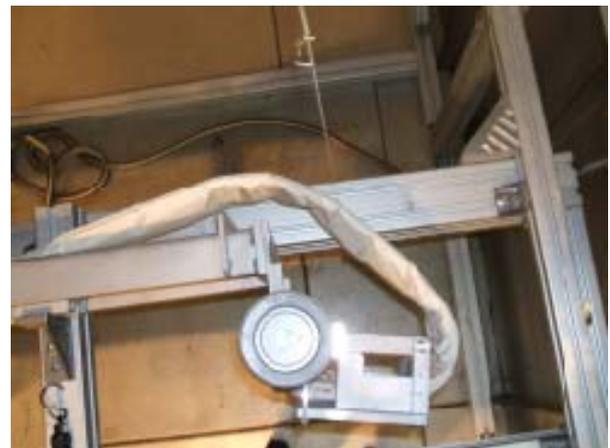
Figure 7: Harness Resistance Test Rig
