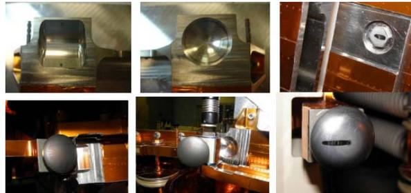
From these it can be seen that the one closest to the secondary pivot, which was a ball on flat surface, had the worst wear - the single wear mark evident in the bottom right hand image. The ECSS for mechanisms states that sliding surfaces should be avoided, this is not always possible.
