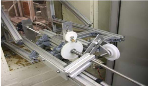
**Figure 8: Harness Resistance Test Rig (Outside Test Chamber)**
