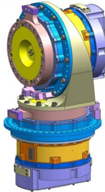
Figure-5 – Type6 Enhanced Pointing Gimbal Assembly
