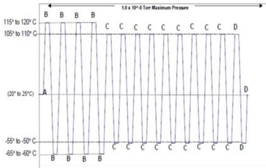
Figure 3 – Temperature Cycling Profile for the 3-Phase design configuration
