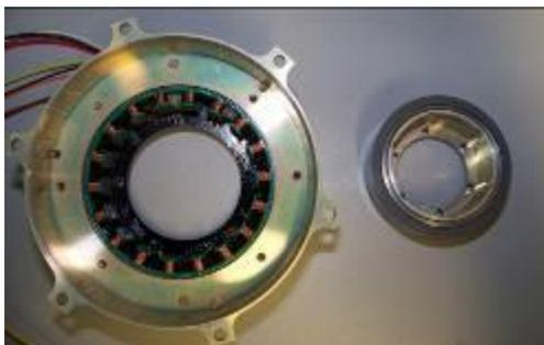
Figure 2. Rotor and stator in the housing of the direct drive motor.
