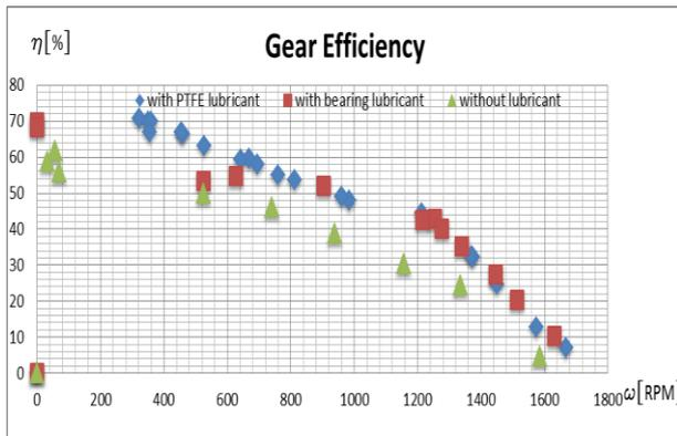
Figure 13. Efficiency via velocity of the input shaft.
