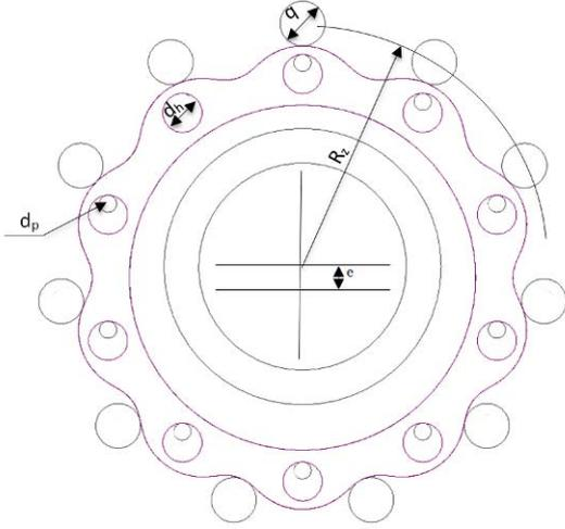
Figure 4. Geometric parameters in the epicycloid one stage gear.
