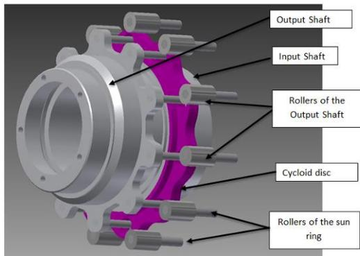
Figure 5. CAD model of the gear used in dynamic simulations.
