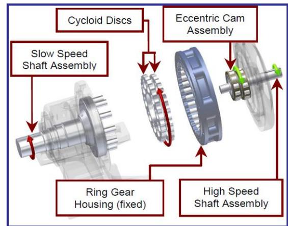
Figure 3. Components of the cycloid gear.
