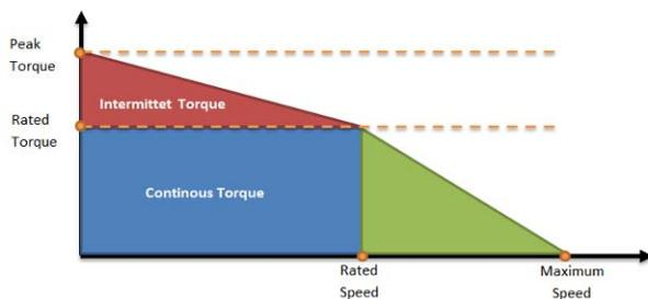
Figure 1. Exemplary torque characteristic via angular speed of the direct drive motor.
