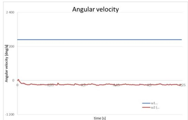
Figure 8. Angular velocity of the components in the cycloid gear.
