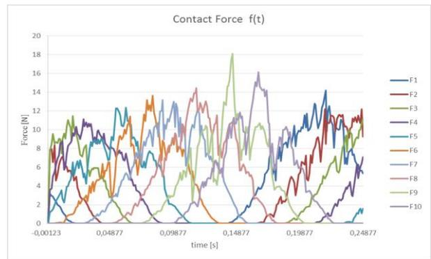
Figure 7. The contact force in the cycloid gear.
