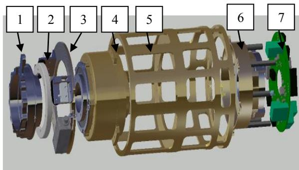
Figure 10. Joint decomposition. 1- output shaft, 2- absolute encoder, 3- end sensor assembly, 4- cycloid gear, 5- housing of the joint, 6- torque motor assembly, 7- control unit.
