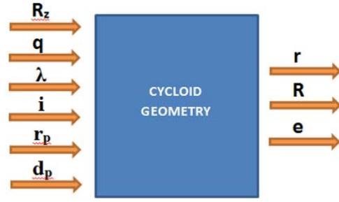
Figure 5. Schematic model of the cycloid gear with marked input and output parameters.  $R_z$ —radius of the arrangement rollers in the sun ring,  $q$ - coefficient of shortened cycloid (radius of the rollers in the sun gear),  $\lambda$ - attitude tooth head to the base,  $i$ - gear ratio,  $r_p$ - radius of the arrangement holes and pins in the low speed mechanism,  $d_p$  - diameter of the pins in low speed mechanism.
