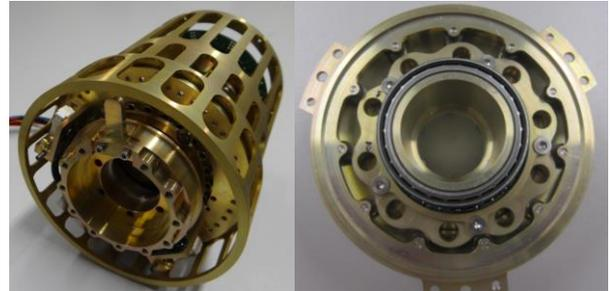
Figure 11. On the left first prototype of the lightweight joint. Picture on the right presents one stage of the cycloid gear.
