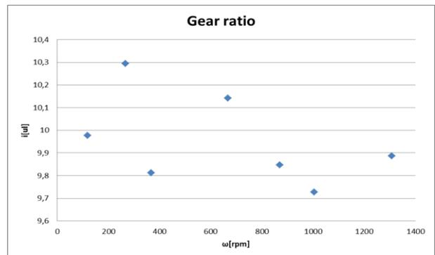
Figure 14. Gear ratio of the one stage reducer as a function of angular speed of the input shaft.
