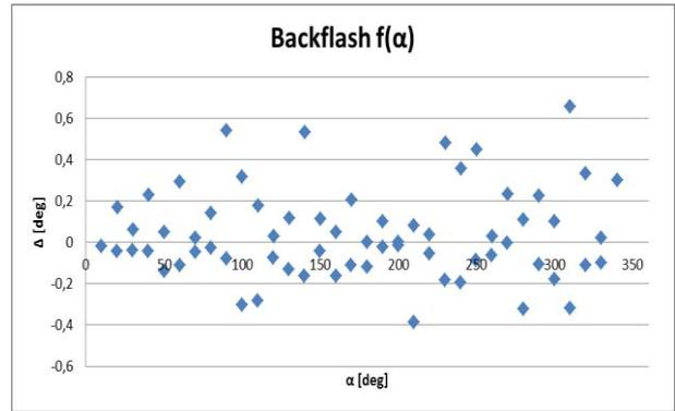
Figure 17. Backlash of the one stage reducer as a function of angular position of the input shaft.
