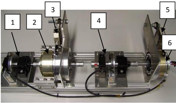
Figure 12. Test bed for dynamic and kinematic characteristic of the cycloid gears. 1- encoder on the output shaft, 2- testing gear, 3- reaction force sensor of the cycloid housing reducer, 4- encoder on the input shaft, 5- reaction sensor of the direct drive housing, 6- direct drive motor.
