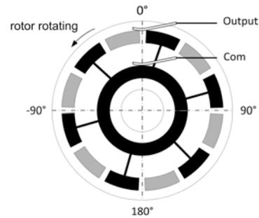
Figure 1. Mechanical representation of the sensor
