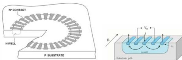
Figure 11. Integrated hall structure
