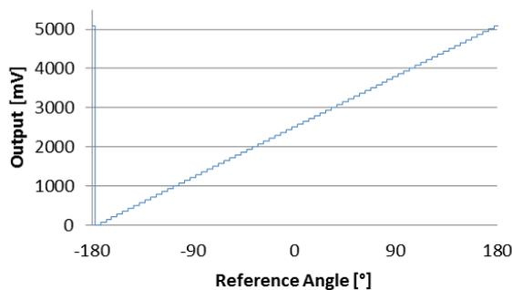
Figure 9. Measured BBM step pot signal
