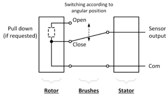
Figure 3. Digital signal electrical diagram
