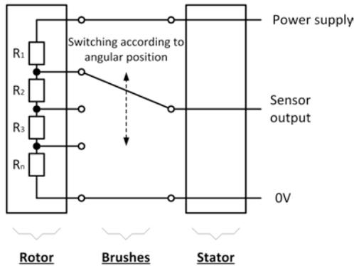
Figure 5. Analog signal electrical diagram
