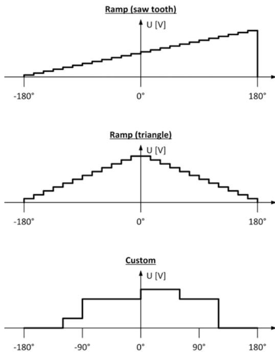
Figure 6. Analog output signals
