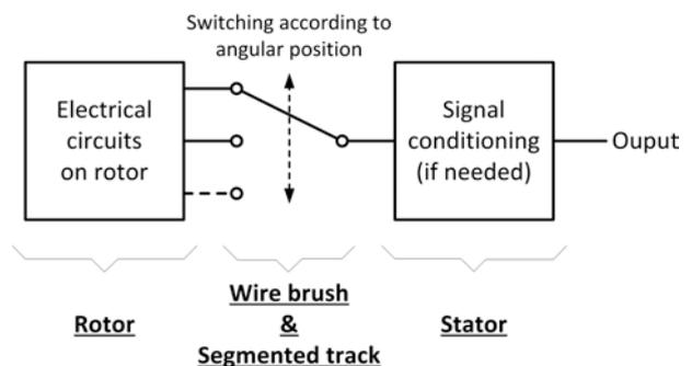
Figure 2. Brushed sensor block diagram
