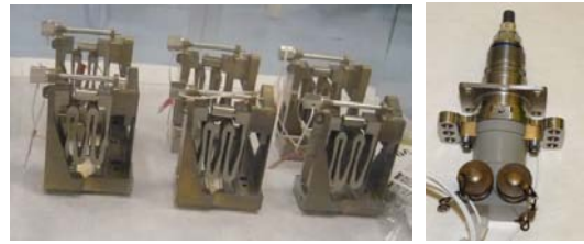
Figure 7. RMA HRM and cartridges
