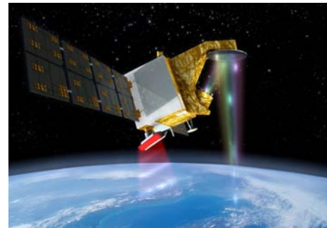
Figure 1. CFOSAT with the SWIM (right) and SCAT (under) instruments
