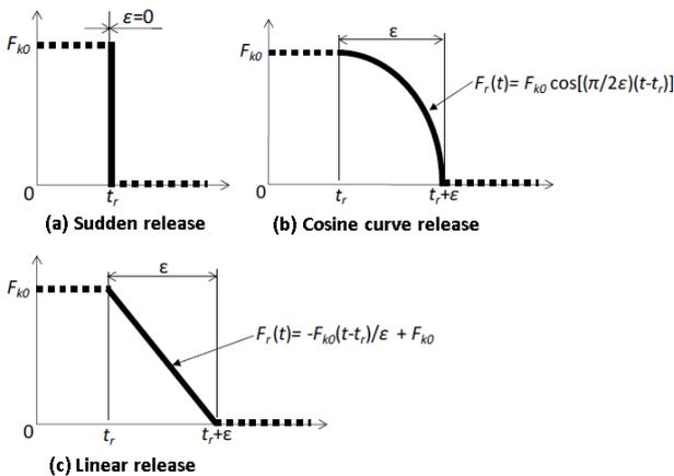
Figure 2. Three types of tension release model.
