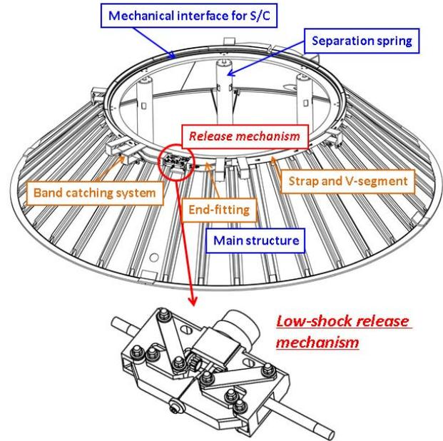
Figure 4. The overview of a payload adapter.
