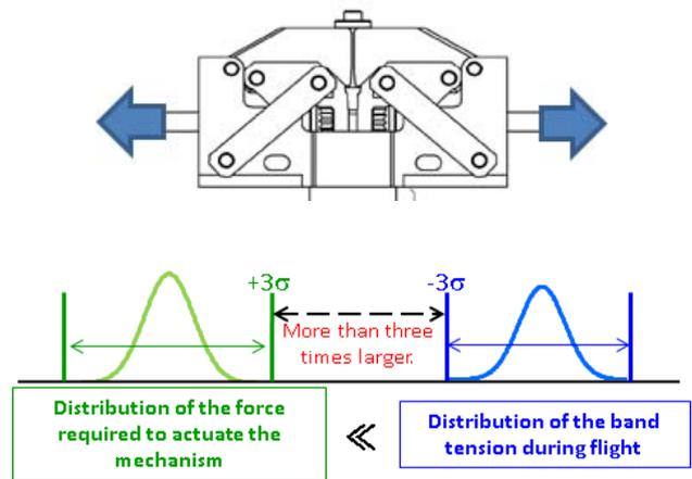
Figure 9. The reliability model of the mechanism.
