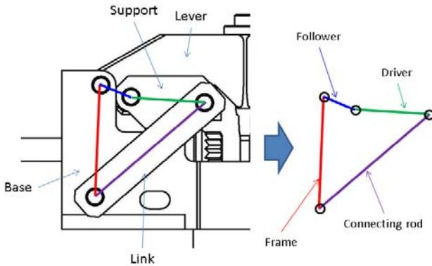
Figure 5. Schematic model as four-bar linkage.
