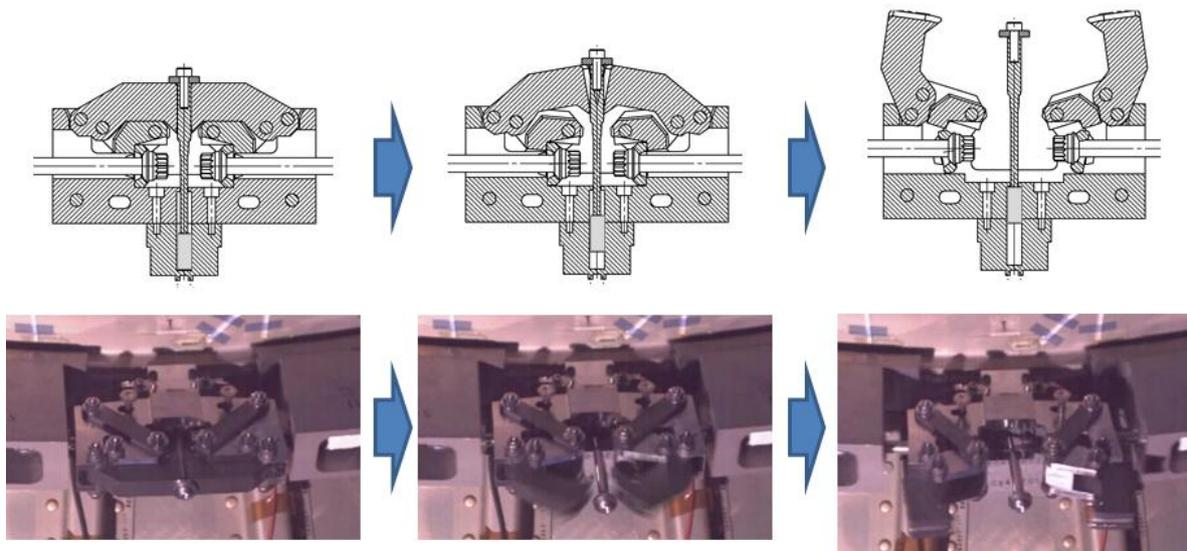
Figure 10. The actuation sequence observed by high-speed video system.
