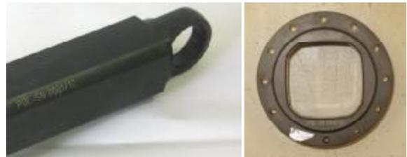
*Tested actuator piston and its anti-rotation bearing using DIN 32712-B P4C profile*
