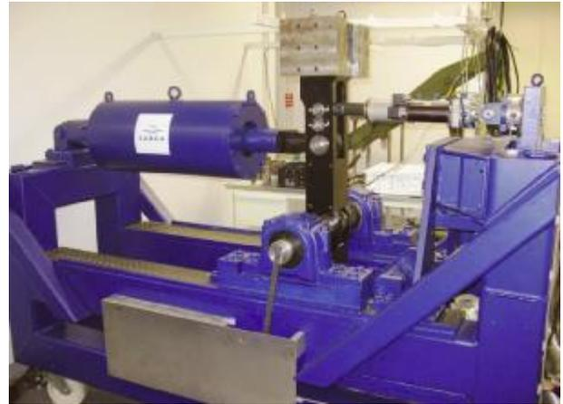
*Inertial load test bench with tested EMA*
