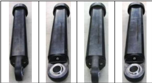
Piston with coating after thermal test with seal retainer coated
