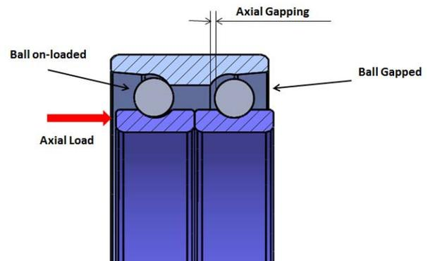
Figure 8. Bearing ball gapping under axial load
