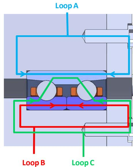
Figure 10. Preload and bearing clamping loops in back-to-back hard-preload configuration
