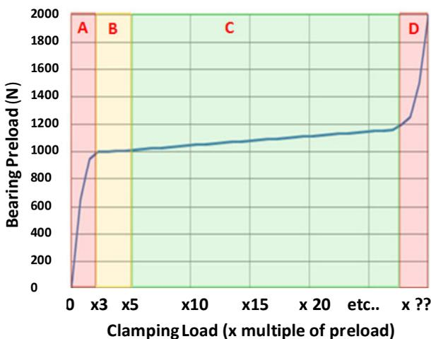
Figure 12 – Assembled preload versus bearing clamping load
