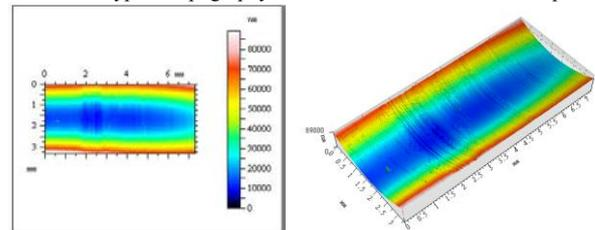
b) 3D surface topography of inside surface of worn flexspline
