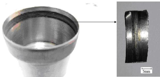
a) Typical topography of inside surface of worn flexspline
