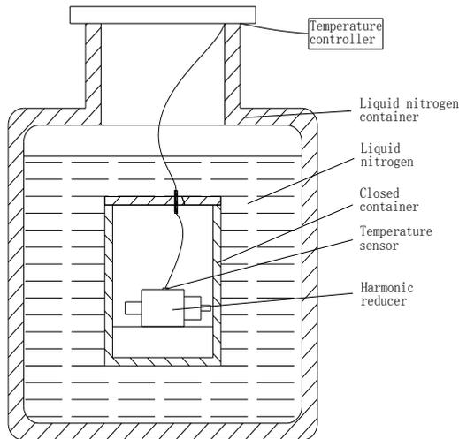
Fig 8 Low temperature storage test of harmonic reducer
