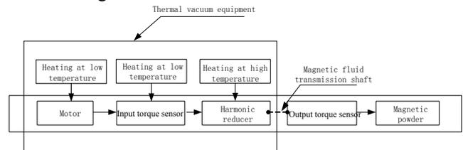
Fig.9 Schematic diagram of the thermal vacuum equipment
