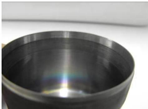
c) innerface of wave generator-flexspline.
