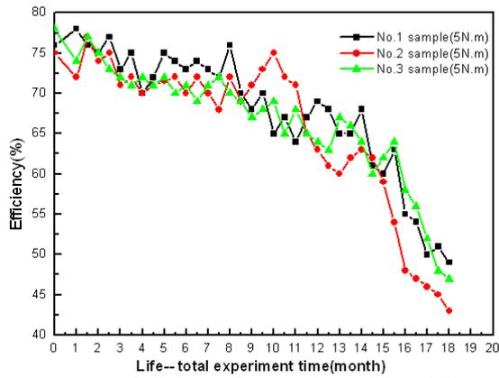
a) curves of efficiency of gears at the condition of 5N.m
