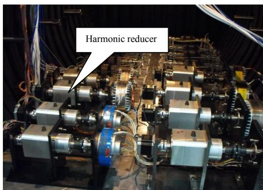
**Fig 1. scene of accelerated tests for harmonic drive gears in vacuum**
