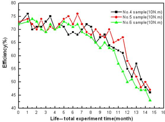
b) curves of efficiency of gears at the condition of 10N.m
