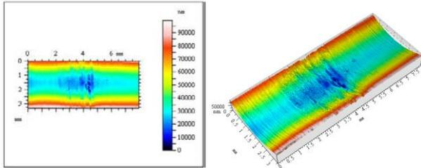
b) 3D surface topography of inside surface of worn flexspline
