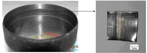
a) Typical topography of inside surface of worn flexspline
