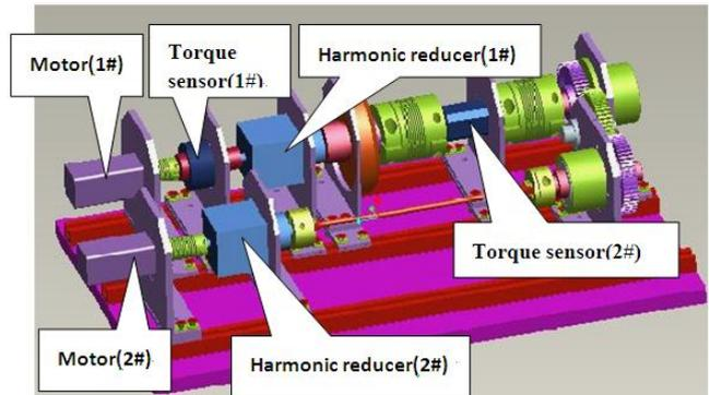
Fig 13 Harmonic reducer performance tester
