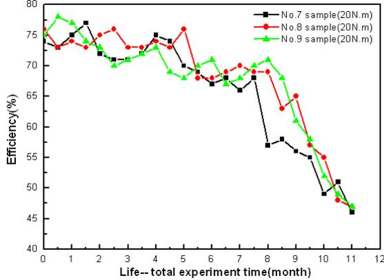
c) curves of efficiency of gears at the condition of 20N.m
