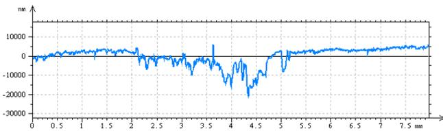
c) Typical scan curve of profile at worn zone
