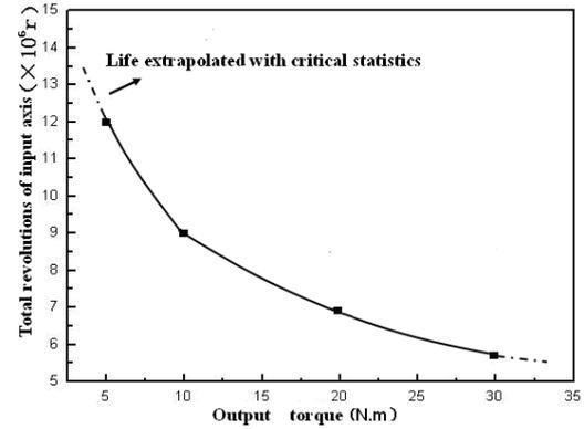
Fig4. Total revolutions of input axis versus output torque
