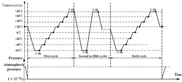
Fig 10 thermal vacuum test profile of harmonic reducer
