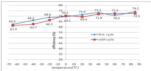
Figure 12 Transmission Efficiency from -65 °C to +85 °C during 1<sup>st</sup> cycle and 6<sup>th</sup> cycle
