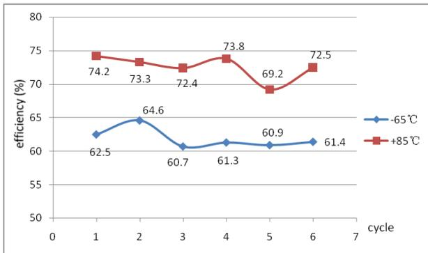
Figure 11 Transmission efficiency at high and low temperature during each cycle
