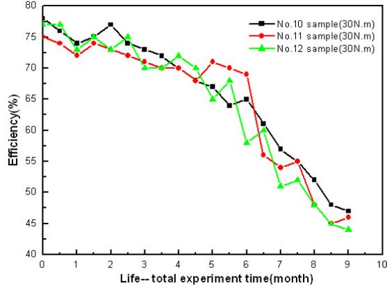
d) curves of efficiency of gears at the condition of 30N.m
