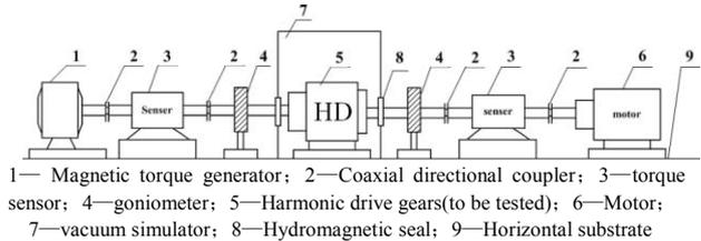
**Fig2. Schematic diagram of performance test for harmonic drive gears**
