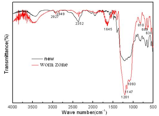
a) FTIR analysis of remnant grease on worn flexspline
