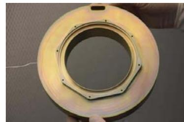
Figure 4. Converter PCB Enclosure – This component also serves a secondary purpose as the upper-outer bearing clamp, and a tertiary purpose as the upper debris containment void and labyrinth seal.
