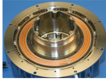
Figure 11. Rotary Transformer primary mounted
