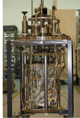
Figure 7. Assembled life test rig with MLI and Thermal Vacuum chamber lid. Upper radiator disc is visible with heat dissipating resistors.
