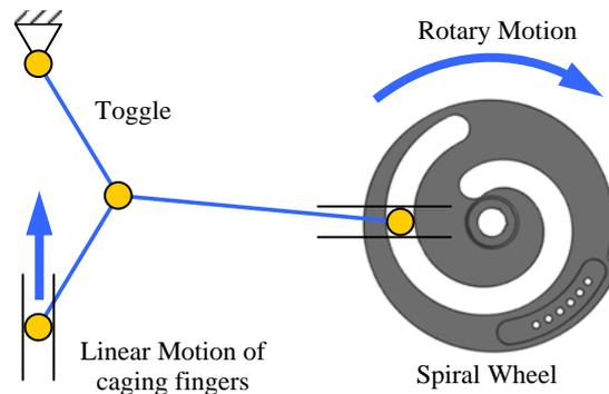
Figure 6. Spiral Cam Principle
