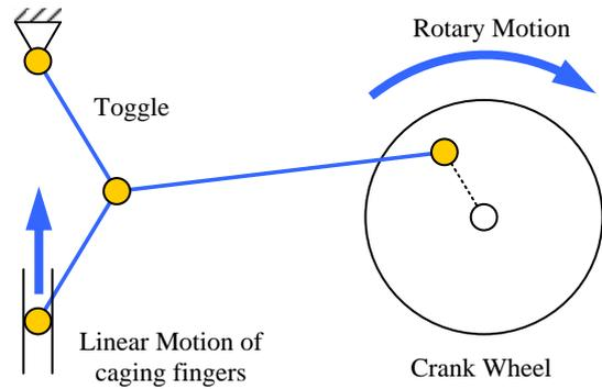
Figure 5. Crank Principle
