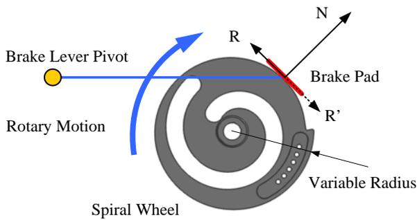
Figure 7. Brake Principle
