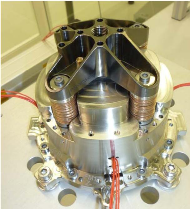
*Figure 3. Transmission Stage Flight Model*
