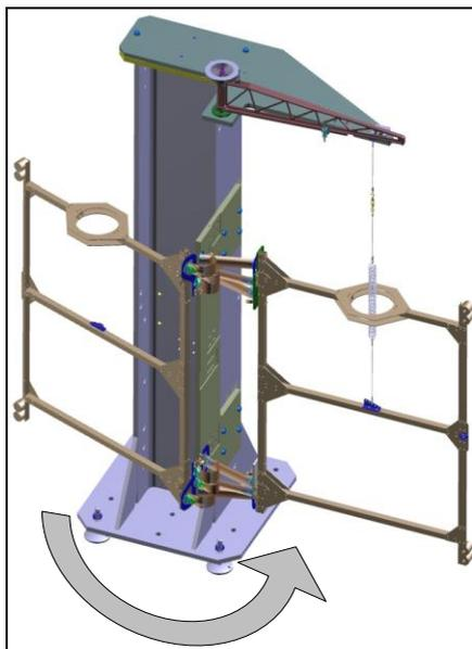
Figure 6. Deployment test stand (start & end position)
