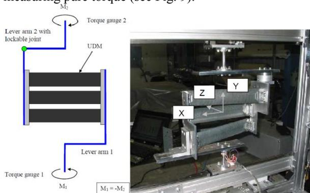
Figure 9. Torque measurement setup
