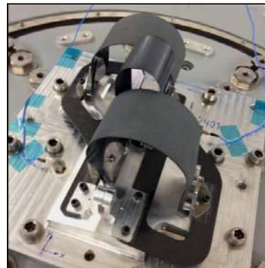
Figure 7. UDM in bent configuration on shaker
