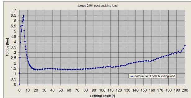
Figure 10. Torque angle relationship of a single UDM
