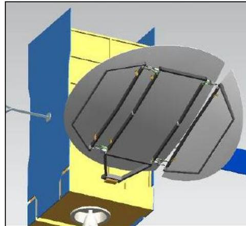
Figure 1. Reflector antenna with sections
