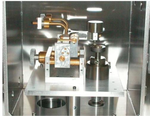
Figure 3. Vacuum pin-on-disc tribometer
