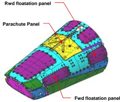
Figure 2. Parachute and floatation panels location
