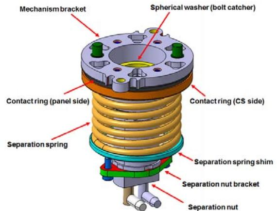
Figure 4. Floatation mechanism concept
