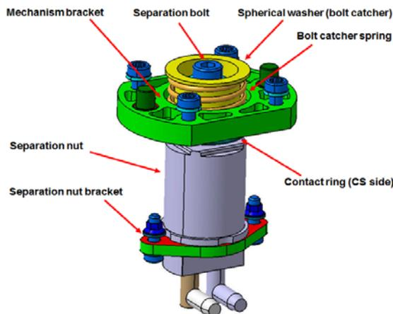
*Figure 6. Parachute mechanism concept*
