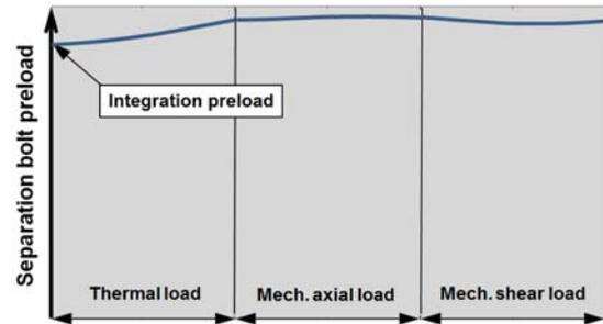
*Figure 7. Separation bolt preload variation*
