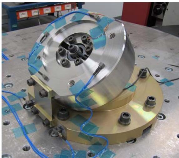
*Figure 13. Vibration test setup*
