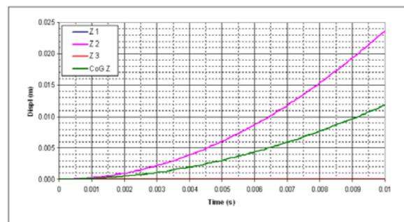
*Figure 8. Front floatation panel corners displacement*
