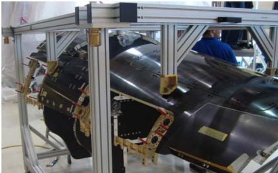
Figure 20. Left floatation mechanisms
