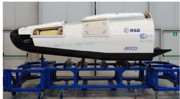
*Figure 18. IXV mock-up for drop test (Courtesy of Thales Alenia Space Italy)*
