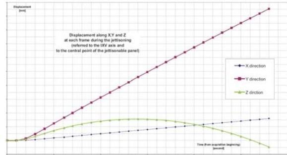
*Figure 16. Front panel trajectory – displacement (Courtesy of Thales Alenia Space Italy)*
