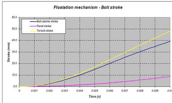
Figure 9. Separation bolt dynamic analysis
