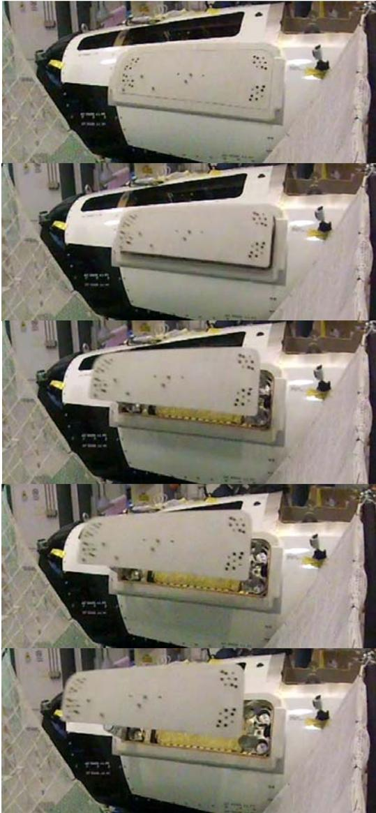
*Figure 15. Front panel release test (Courtesy of Thales Alenia Space Italy)*
