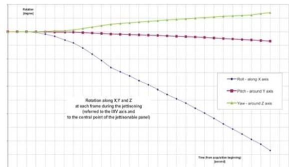
*Figure 17. Front panel trajectory – rotations (Courtesy of Thales Alenia Space Italy)*
