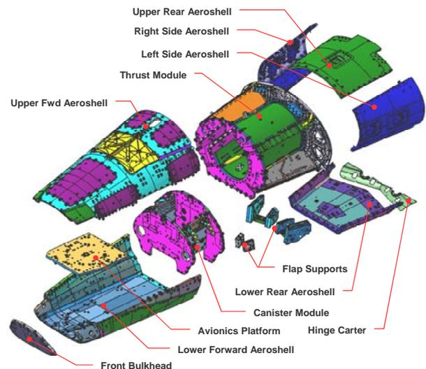
*Figure 1. Monocoque design concept*
