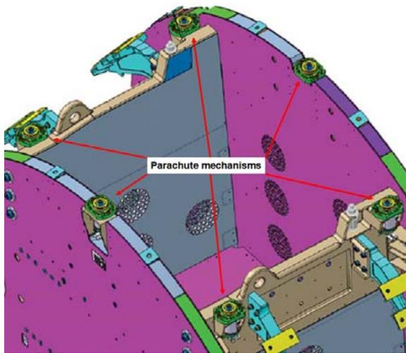
*Figure 5. Parachute mechanism layout*
