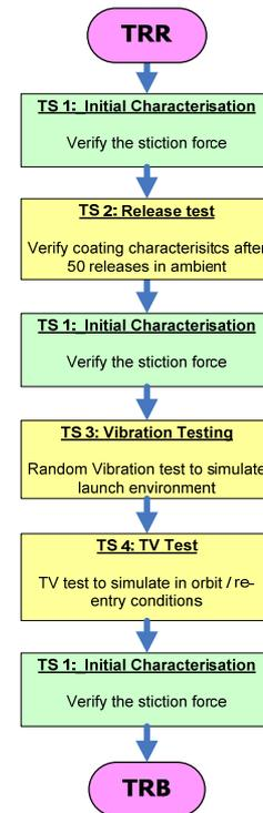
Figure 10. Qualification test flow (mechanism level)
