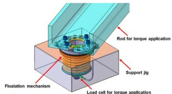
Figure 11. Rotation test setup
