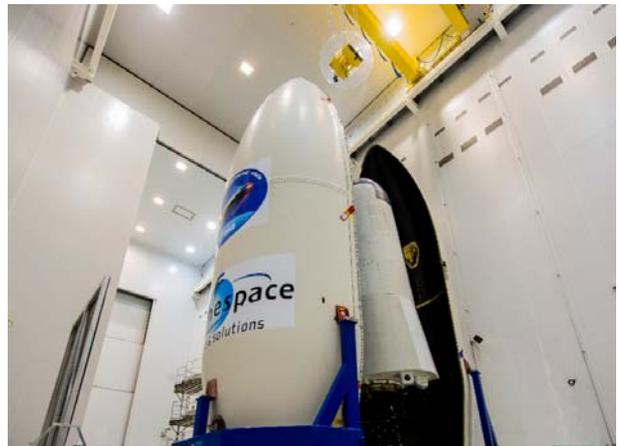
Figure 22. IXV during Vega fairing encapsulation (photo: ESA)
