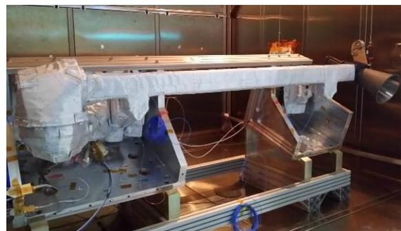
Figure 2 MGAMA: APM, boom and horn
