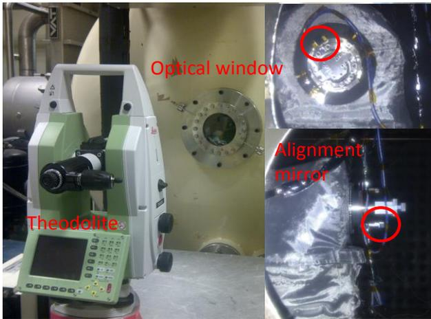
Figure 6 Theodolite, window and alignment mirror
