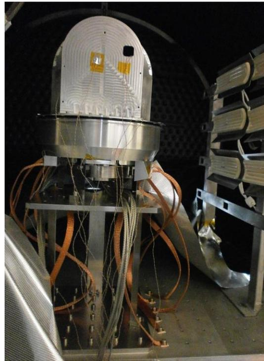
Figure 7 Isostatic support, thermal braids and IR lamps
