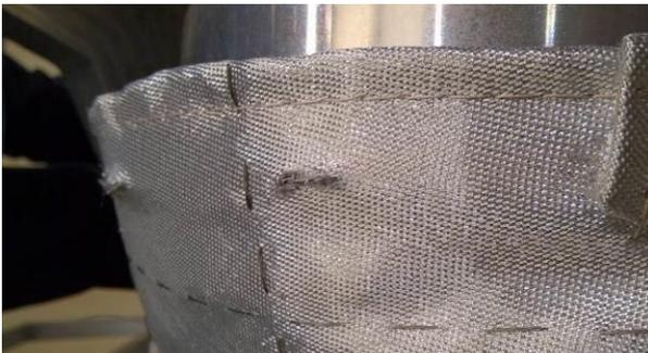
Figure 13 Damaged area of MLI in the contour
