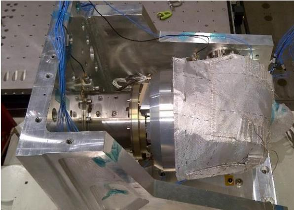
Figure 12 HGA APM vibration test
