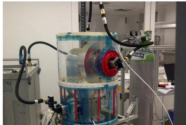
Figure 15 . Purged movable enclosure with RF ports
