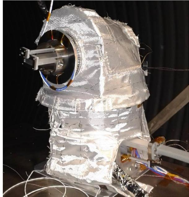
*Figure 3 HGA EQM APM in TV test configuration with MLI and RF loads and input Waveguides*
