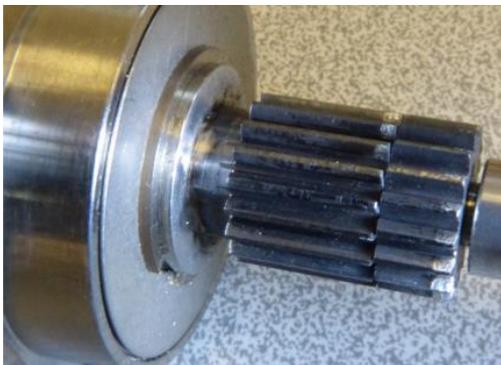
Figure 18 . Azimuth output pinion (main & anti-backlash) wear pattern
