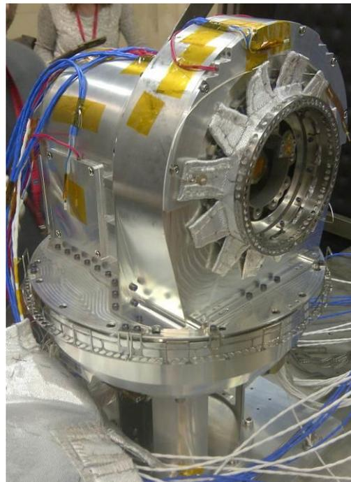
*Figure 4 HGA APM instrumented with heater plates and thermistors outside the shield*
