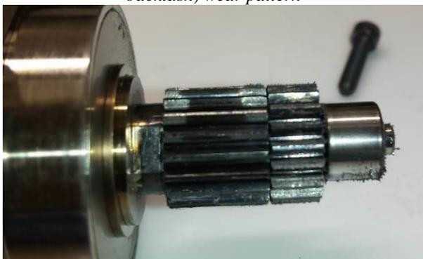
Figure 1. Elevation output pinion (main & anti-
