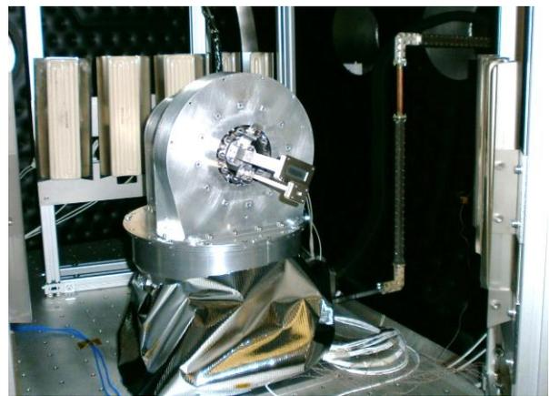
Figure 5 HGA PFM in TV test with IR lamps and fixed Ka waveguides
