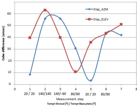
Figure 9 APM Thermal distortion between different measurement temperatures
