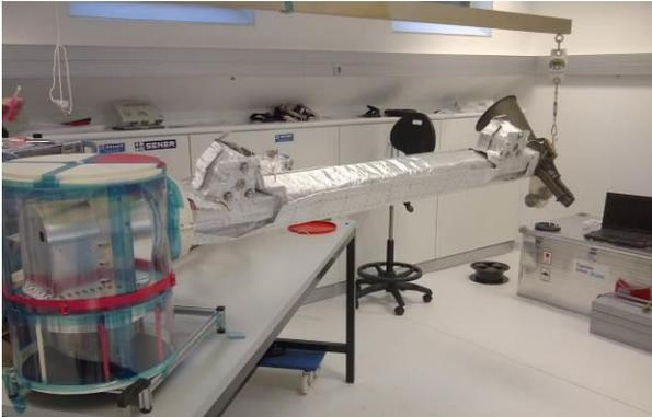
Figure 16 . Movable purge box for MGAMA during functional test with zero-g
