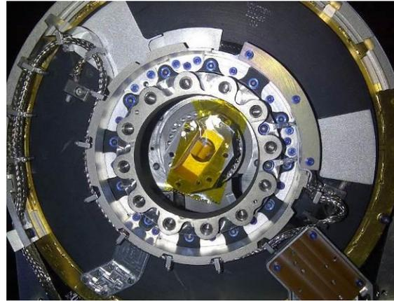
Figure 10 MGA Twist capsule after contact with switch assembly
