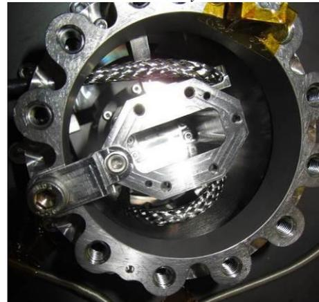
Figure 11 Hollow shaft elevation twist capsule
