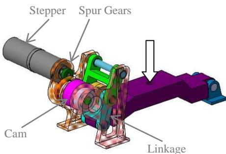
Figure 7. - Stepper+ Cam +Linkage detail
