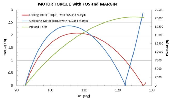
Figure 17.- Motor Torque with ECSS factors
