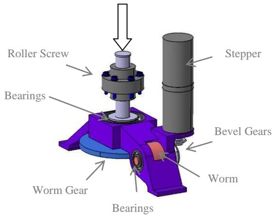
Figure 5.- Stepper+Gears +Centered Roller Screw
