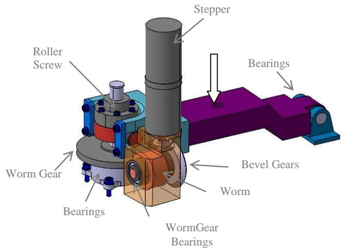
Figure 4.- Stepper+Gears +Lateral Roller Screw
