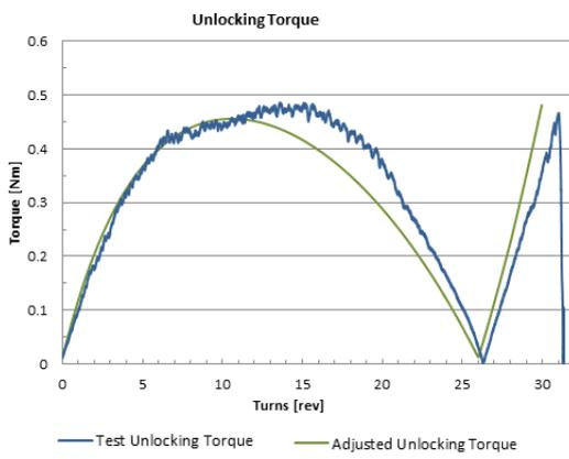
Figure 15.- Unlocking Torque Adjustment
