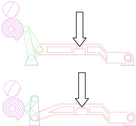
Figure 6.- Stepper+ Cam +Linkage
