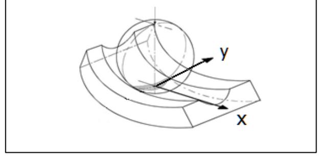
Ball on raceway contact:  $\kappa > 1$
