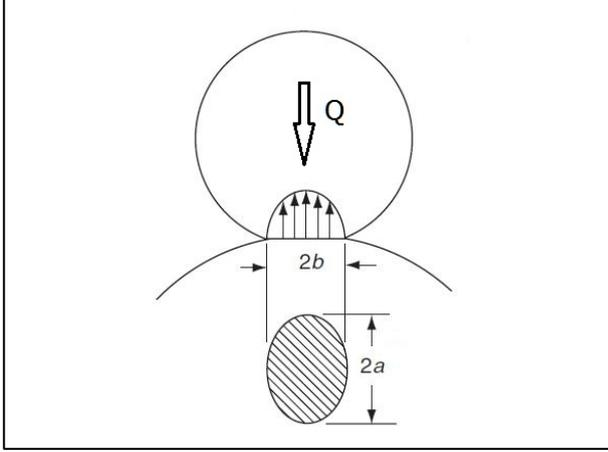
Figure 1 - Hertzian pressure and deformation
