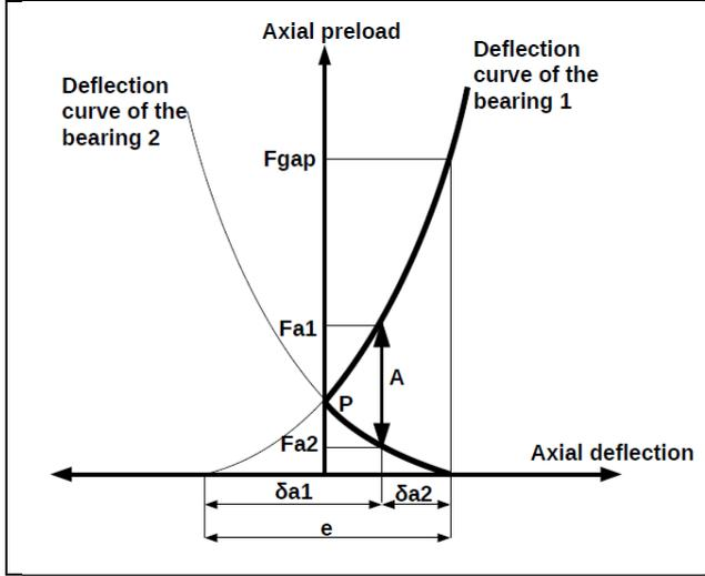
Figure 5 – Deflection curve of a paired bearing
