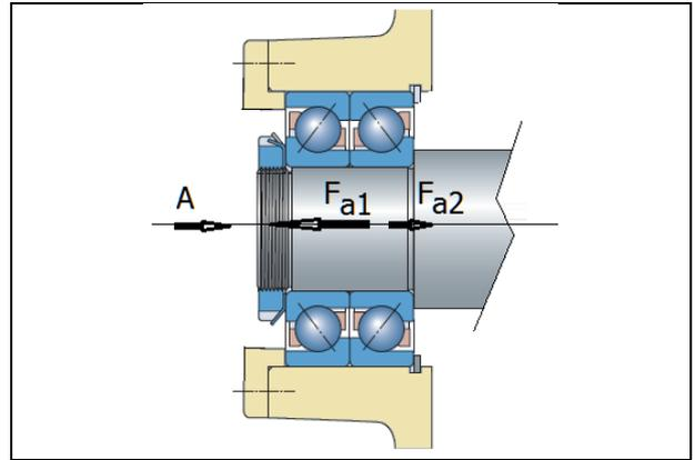
Figure 4 – Preloaded bearing submitted to an axial load
