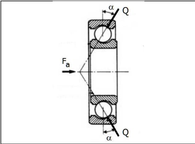
Figure 3 - Axial loading of an angular contact bearing
