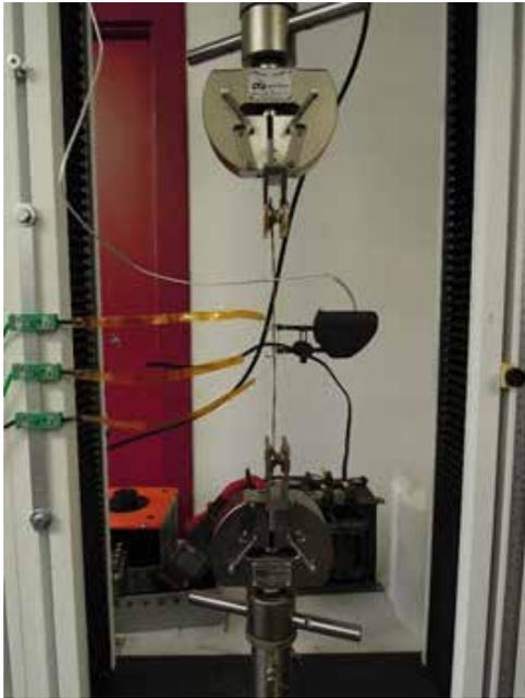
Figure 2 - Test bench used for thermal cycling of pre-stressed single crystal samples
