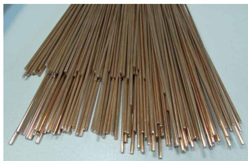
Figure 1 - Cu-Al-Ni single crystal Ø2.2 mm wires made with special Nimesis process
