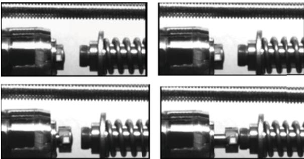
Figure 11. An example of a sequence of movements (presented: the 5th power setting; the time difference between each frame is 0.53ms). On the left: a blocked counter-mass with a protruding hammer inside; on the right: the test stand hitting rod. The thread above the scene is a scale reference – this is a standard M8 thread.
