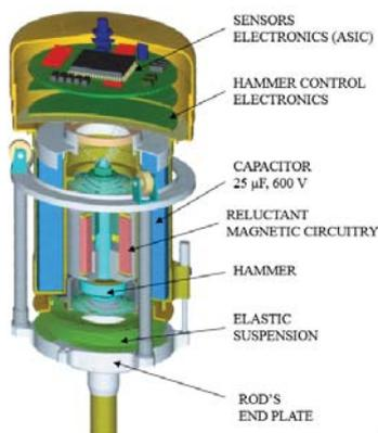
Figure 1. MUPUS insertion hammering device with an electromagnetic drive.
