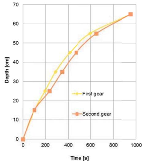
Figure 18. Dependence of time imbedded from depth in Syar regolith analogue.
