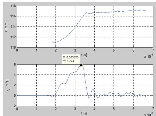
Figure 14. Velocity plot for power setting -3, measured velocity before hit.
