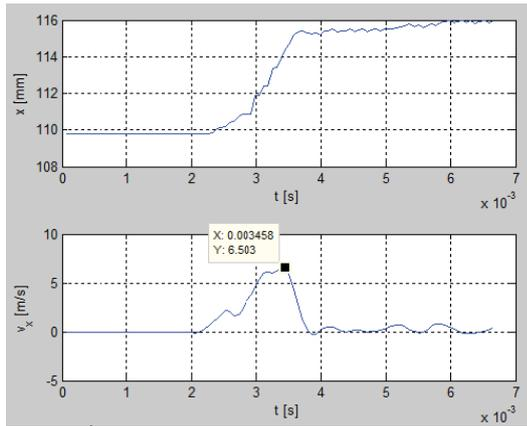
Figure 15. Velocity plot for power setting -4, measured velocity before hit.
