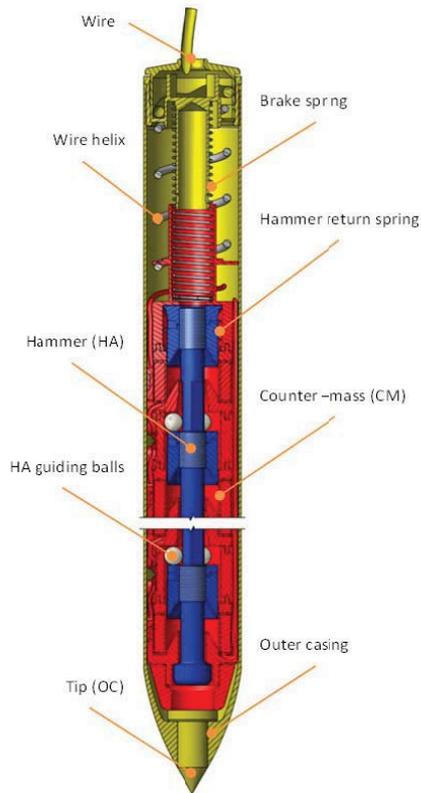
Figure 7. EMOLE CAD model cross-section.
