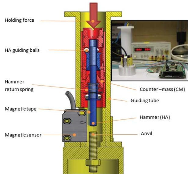
Figure 4. Verification test-stand (with 'foot'), in the top right the actual stand with control electronics.
