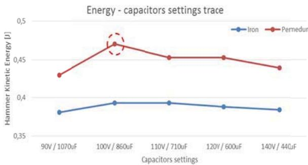
Figure 5. Constant stored capacitor energy is maintained – 4.3J. Plot represents resulting kinetic energy of the hammer as a function of different capacitor settings for Iron and Permendur 49 coils. Dashed circle indicates optimal capacitor settings (concerning the stroke energy as the optimization criteria).
