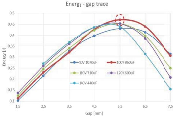
Figure 6. Optimization of Hammer travel gap. Plot represents measured kinetic energy of the hammer for Permendur 49 coil for the selected capacitor energy level (4.3J). Dashed circle indicates resulting optimal gap for the selected capacitor settings.
