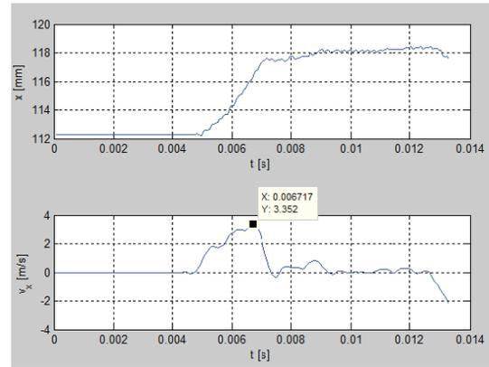
Figure 12. Velocity plot for power setting-1, measured velocity before hit.
