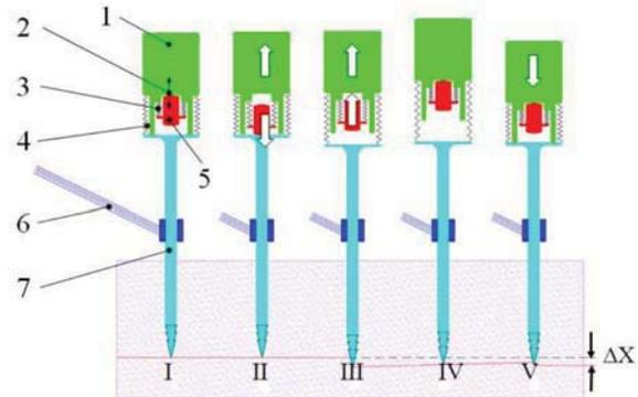
Figure 2. Principle of operation of the penetrator MUPUS (main parts: 1 - counter-mass; 2 - place to generate power; 3 & 4 - spring suspension; 5 - hammer; 6 - manipulator arm (1m) ending lead clamp (0-1N); 7 - hammered rod)
