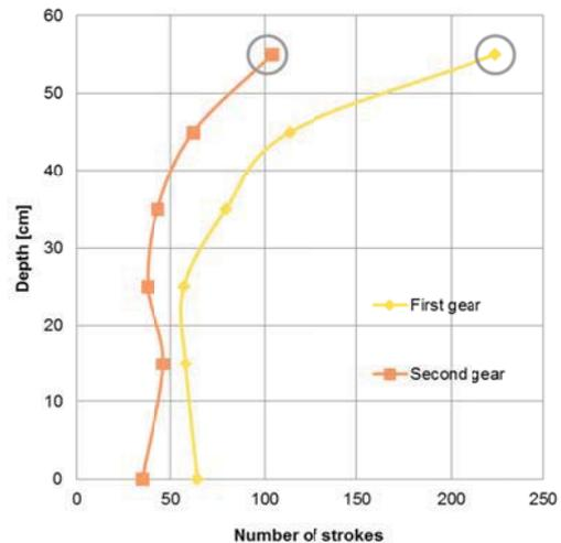
Figure 19. Dependence of number of strokes from depth in Syar regolith analogue. Numbers of strokes are presented for 10 cm depth sections and only first one is for 15 cm.
