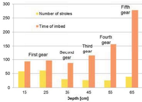
Figure 20. Dependence of number of strokes and time of imbed from depth for five power settings. EMOLE needed more stroke on higher power levels to reach the next ten centimeters because, the bottom volumes of the regolith were more much more compressed.
