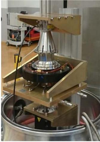
**Figure 4: Bearing Characterization Test Set-up in a TV chamber**
