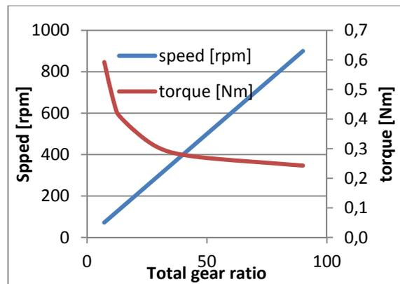
Figure 2: Motor speed & Motor torque vs. gear ratio
