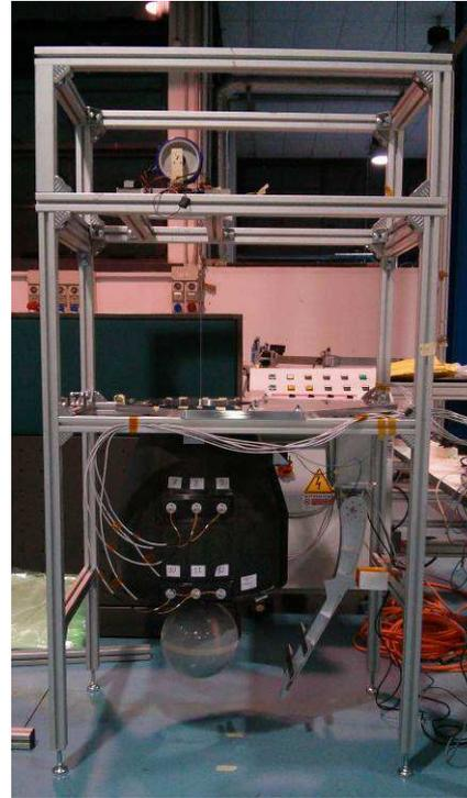
Figure 5. 0-g Ground Support Equipment (GSE).
