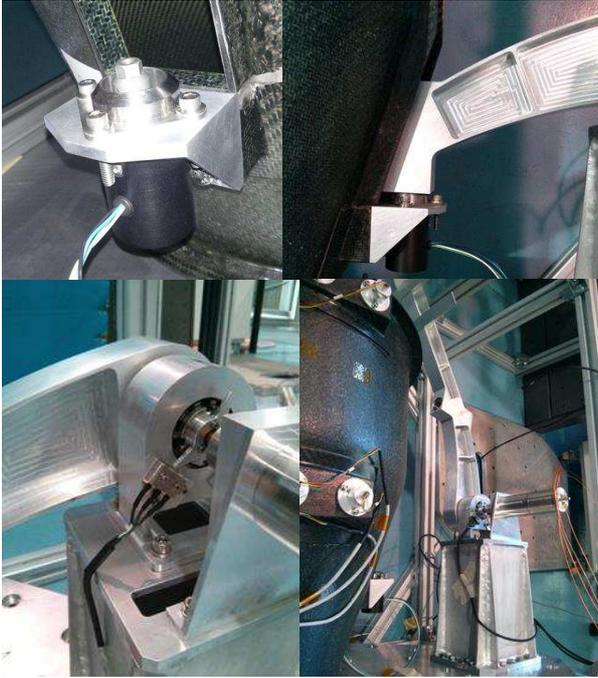
Figure 4. from top-left: HDRM, arm latching, arm hinge, arm and support tower.
