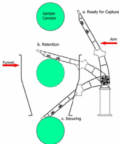
Figure 1. SCCM Operative modes: a. Ready for capture, b. Retention, c. Securing.
