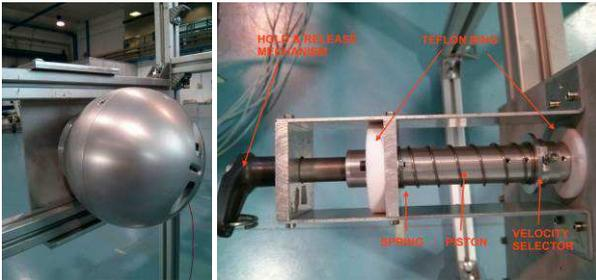
Figure 9. OS Launcher.
