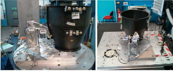
Figure 8. VT setup shaker (left) and slip table (right).
