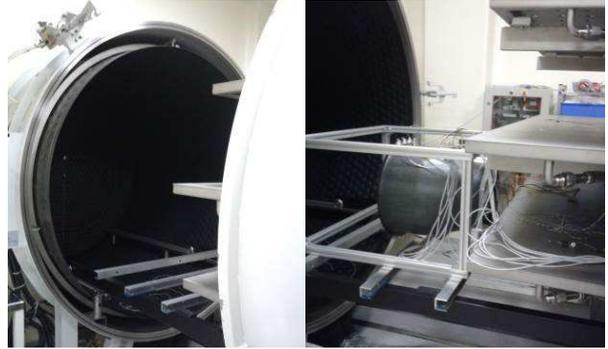
Figure 7. T-V test setup.
