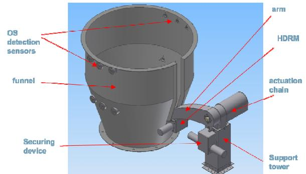
Figure 2. SCCM flight model concept.
