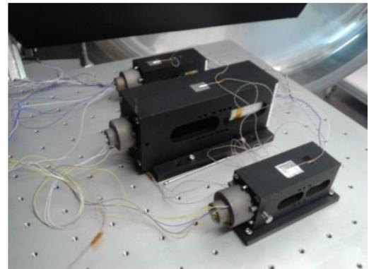
Figure 17. Setup for thermal vacuum tests of Pin Puller.
