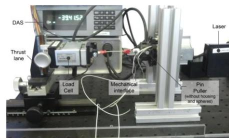
Figure 9. Measurement of pin friction of pin puller.
