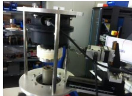
Figure 8. Measurement of resistive torque of REACT.
