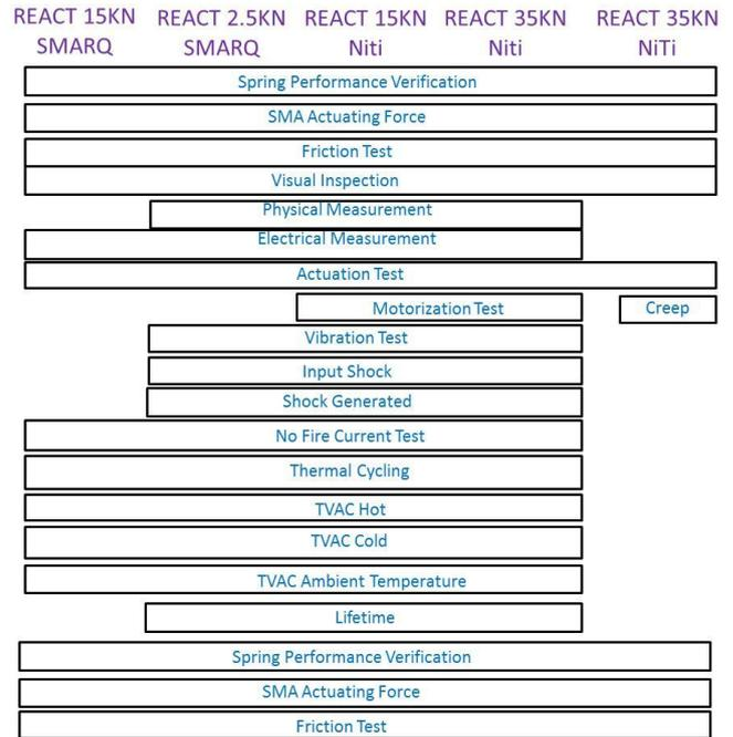
Figure 5. Test sequence of the proposed qualification campaign.
