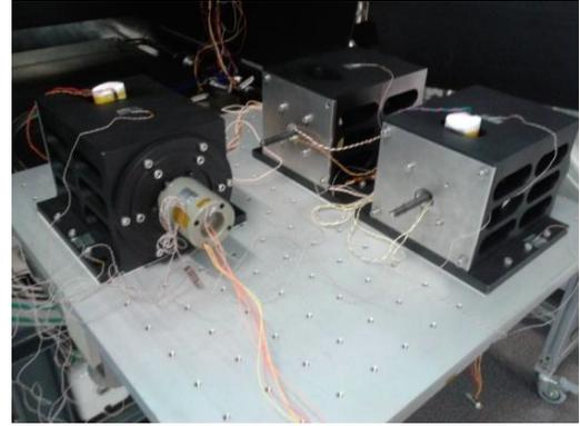
Figure 16. Setup for thermal vacuum test of REACT.
