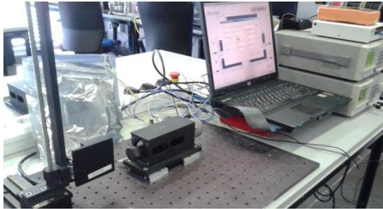
Figure 11. Setup for Pin Puller actuation.
