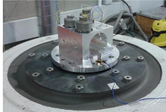
Figure 12. Axial vibration of Pin Puller.
