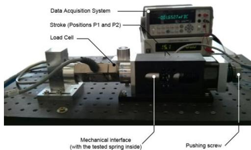
Figure 7. Measurement of spring performance.
