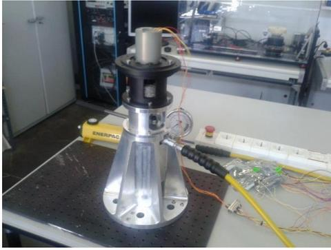
Figure 10. Hold down stack for REACT actuation.
