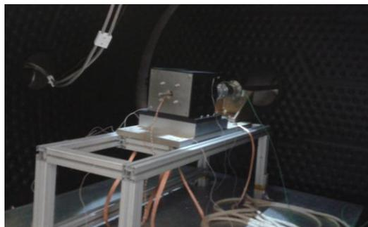
Figure 18. Measurement of resistance torque of REACT Crown in thermal vacuum.
