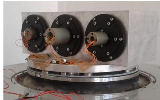
Figure 13. Radial vibration of REACTs .
