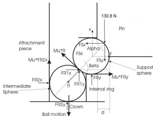
Figure 1. Kinematic scheme of the proposed hold-down and release mechanism.
