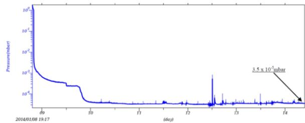
Figure 10. Vacuum levels in respect to time.
