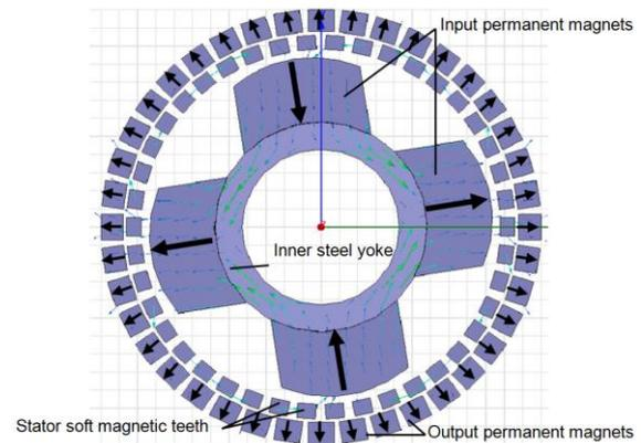
Figure 2. Magnetic configuration of MAGDRIVE prototype.
