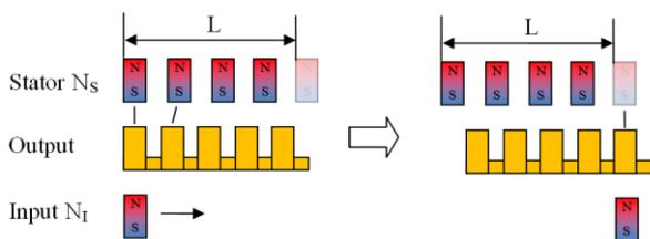
Figure 1. Scheme of the MAGDRIVE mesh principle.
