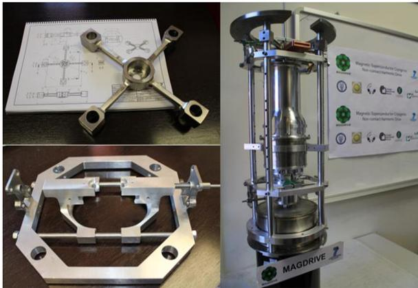
Figure 5. Structural connection (top-left), launch lock mechanism (bottom left) and MAGDRIVE assembled (right).
