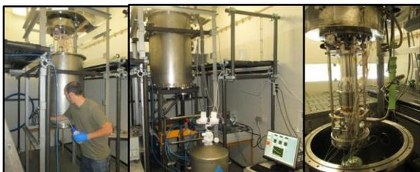
Figure 6. MAGDRIVE integrated in the vacuum chamber.
