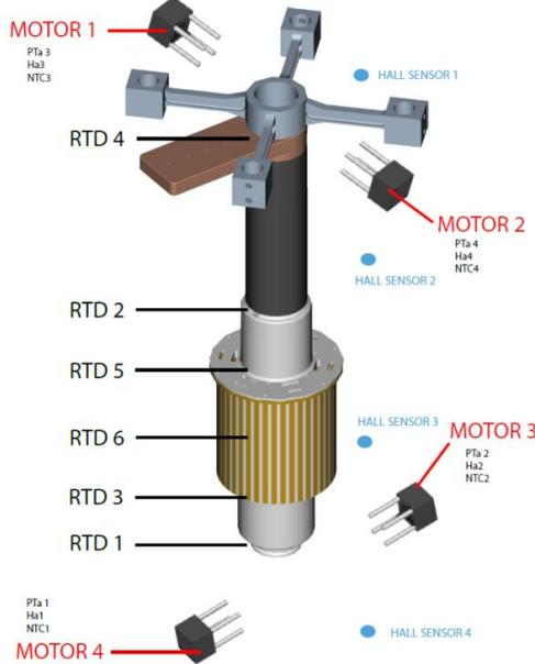
Figure 8. Internal location of the temperature and magnetic field sensors.
