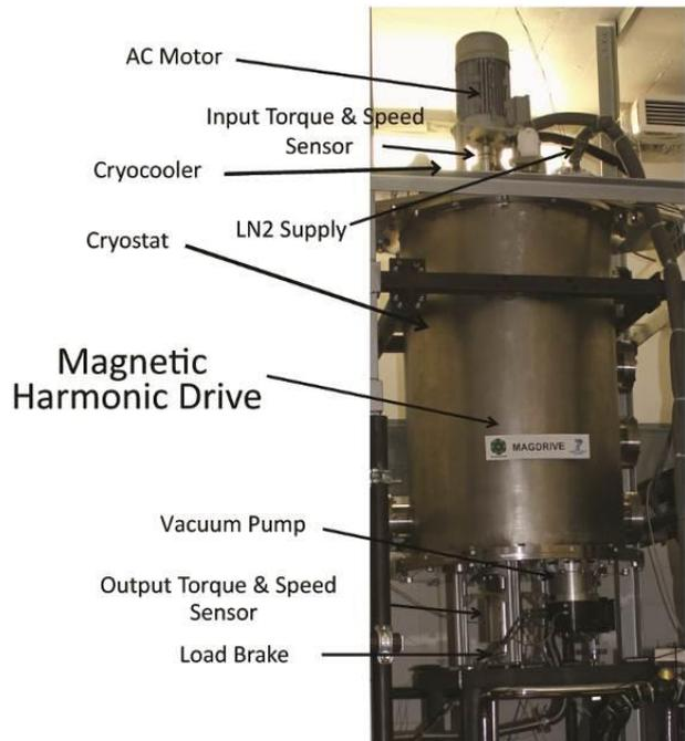
Figure 7. External assembly of the test.
