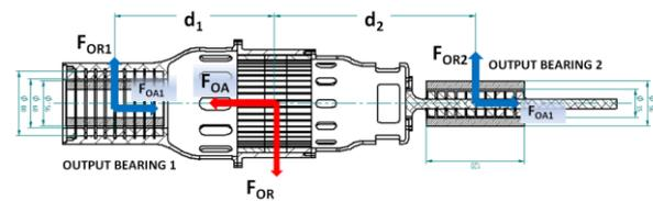
Figure 4. Superconducting magnetic bearing output design.
