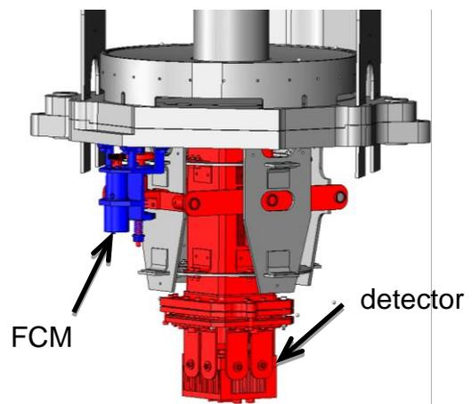
Figure 2. Focus mechanism location within camera.
