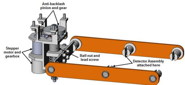
Figure 3. Focus mechanism.
