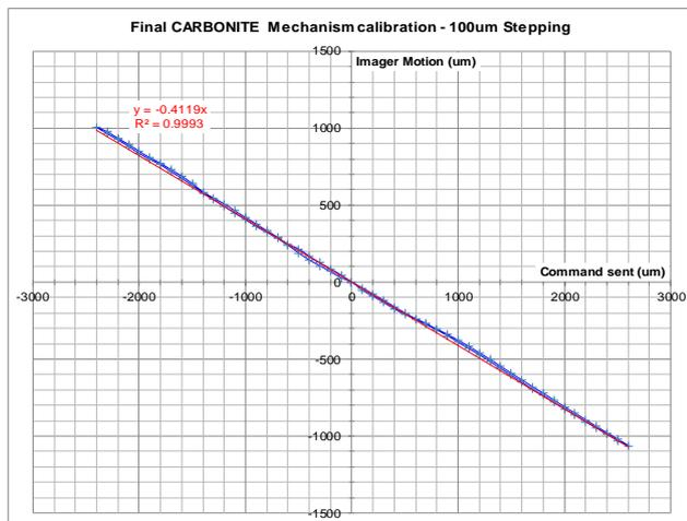
Figure 5. Focus mechanism linearity
