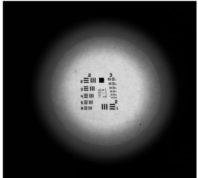
Figure 6. Focus measurement
