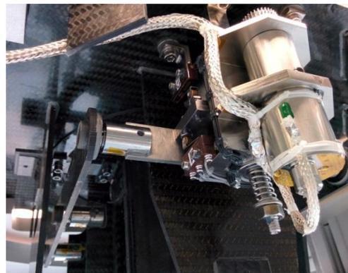
Figure 4. Focus mechanism integrated to camera.
