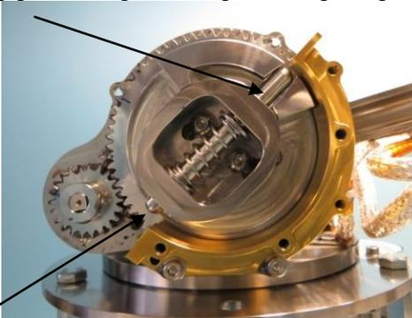
pin is no longer constrained by housing, hinge shaft is free to rotate
