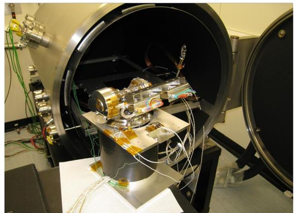
Figure 12. BSADM TVAC Test Setup
