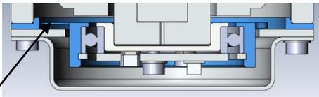
Bearing membrane allowing for axial translation of rear bearing
