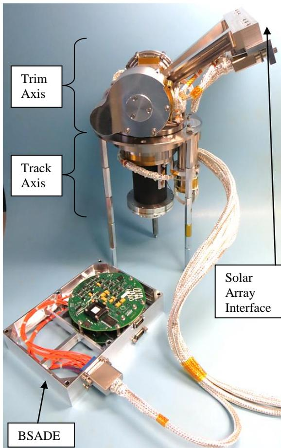
Figure 4. BSADA (BSADM and BSADE)
