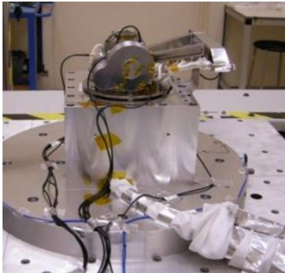
Figure 9. BSADM Vibration Test Setup
