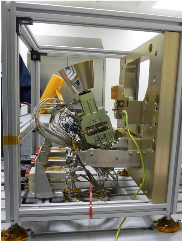
*Figure 5 Test of the fail safe function of the SCM QM assembly*
