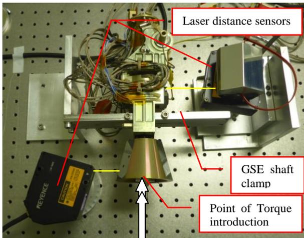
Figure 9 setup to investigate soundness of interface wheel to shaft
