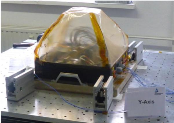
Figure 7 SCM on ringing table (shock test)
