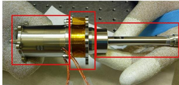
Figure 2 SCM drive unit (motor, gear, bearing & shaft)
