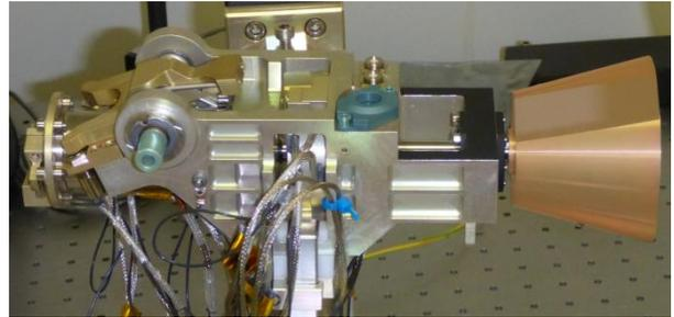
Figure 1 SCM with dummy wheel (right), cone and axis mechanical interfaces
