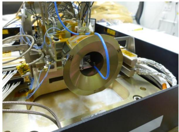
*Figure 6 Central acceleration sensor at mirror wheel interface*
