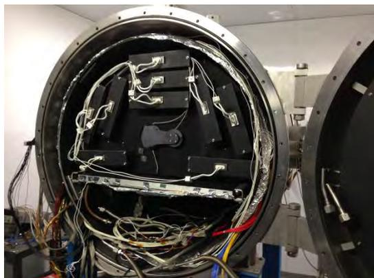
Figure 11. EQM SOLAR SIMULATION TEST (DM&FT) in chamber
