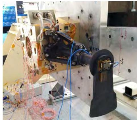
Figure 8. EQM Shock test Z Axis test set up
